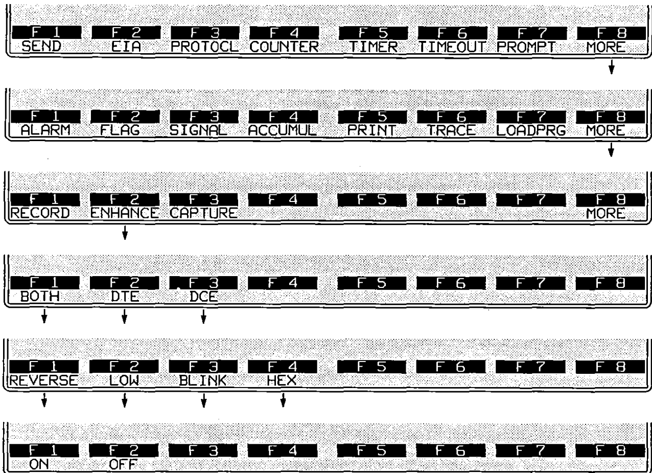
Figure 31-13 Layer 1 enhancements must be turned off as well as on by trigger.
