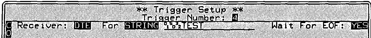
Figure 24-3 Both alphanumeric and hexadecimal characters can be entered as part of a condition search string.
