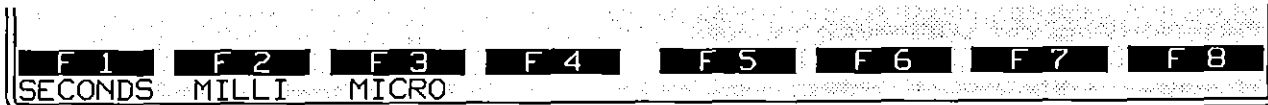
Figure 30-10 After a timer is named for printout display, a new softkey rack allows you to specify unit of time.
