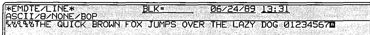
Figure 31-9 The INTERVIEW aborts a BOP frame by closing it with a byte of FF instead of 7E .
