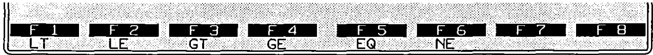
Figure 30-2 A set of relational operators compares the counter value to a user-entered value.
