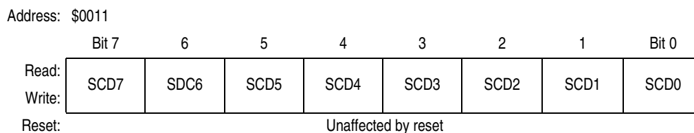
Figure 9-8. SCI Data Register (SCDR)
