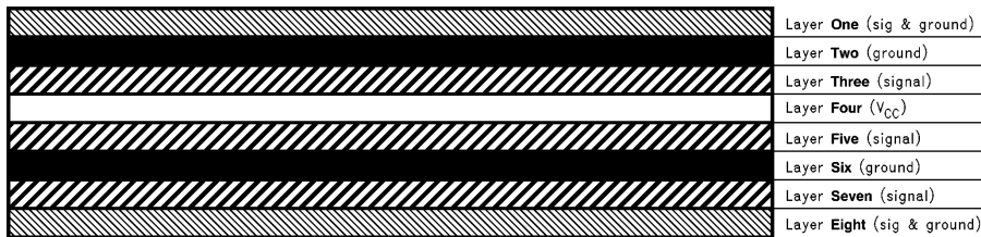
FIGURE 23. Board Layer Assignment Recommendation
