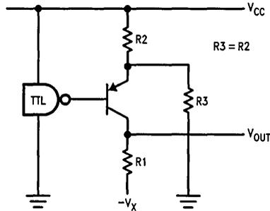
FIGURE 3-23. pnp Transistor Shifting TTL Output
