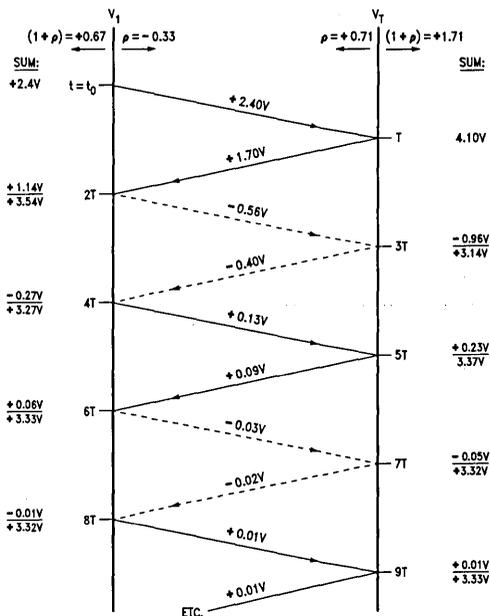
FIGURE 3-9. Lattice Diagram for the Circuit of Figure 3-8
