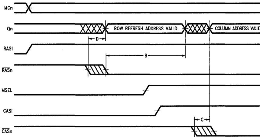
FIGURE 4. Specifications Applicable to Refresh Cycle Timing ( $MC_n = 00,01$ )
