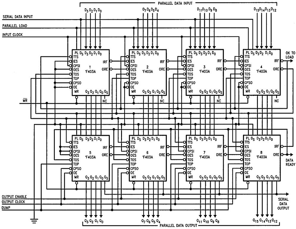
FIGURE 6. A 31 x 16 FIFO Array
