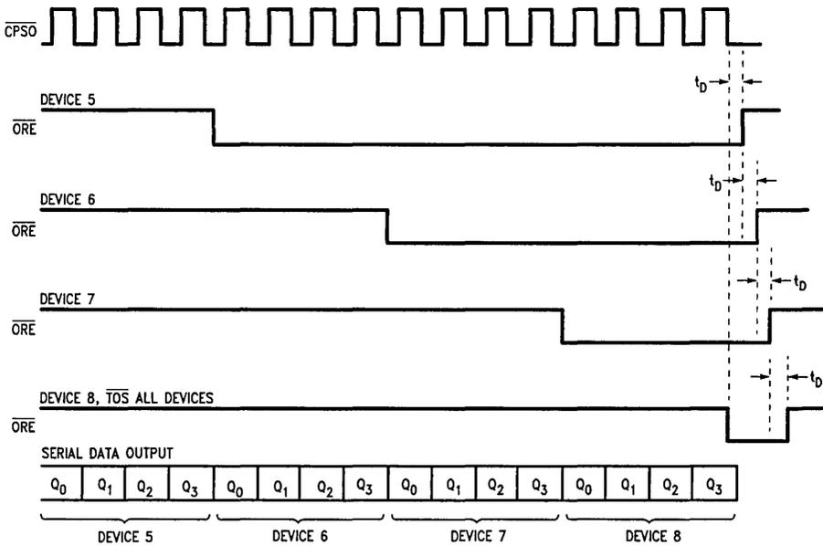
**FIGURE 8. Serial Data Extraction for Array of Figure 6**
