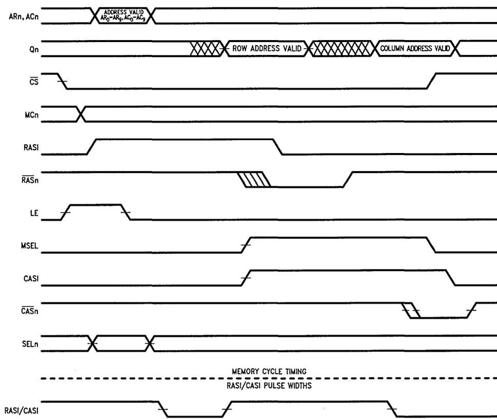
FIGURE 1. Dynamic Memory Controller Timing
