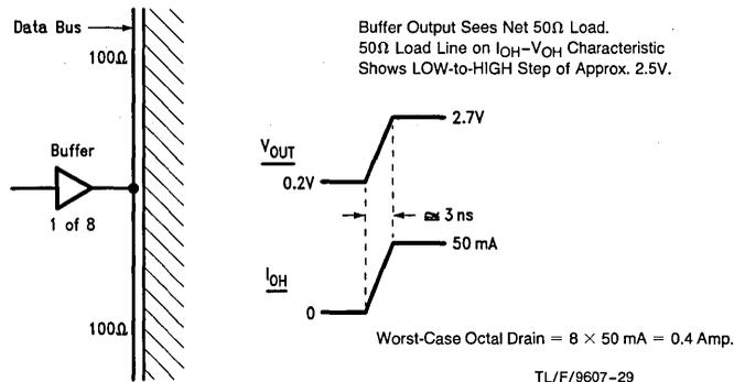
FIGURE 3-15. ICC Drain Due to Line Driving
