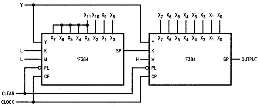
FIGURE C. 12-Bit by n-Bit Twos Complement Multiplier
