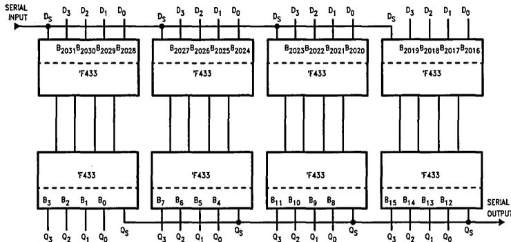
FIGURE 9. Final Position of a 2032-Bit Serial Input
