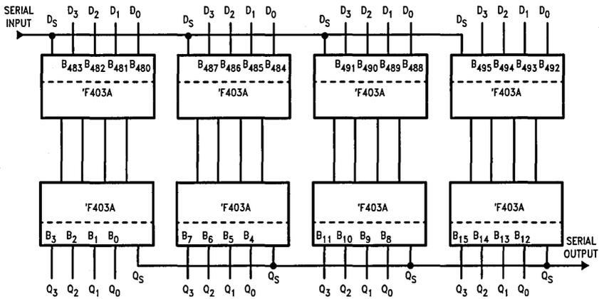
FIGURE 9. Final Position of a 496-Bit Serial Input
