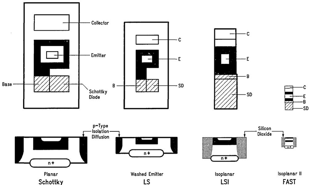
FIGURE 1-1. Relative Transistor Sizes in Various TTL Families
