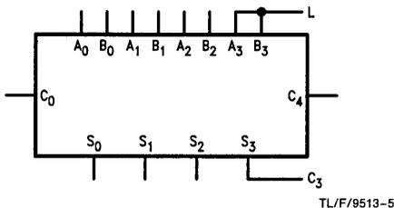
FIGURE 2. 3-Bit Adder
