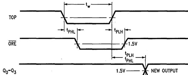
Conditions:  $\overline{IES}$  LOW when initiated,  $\overline{OE}$ ,  $\overline{CPSO}$  LOW; data available in stack
