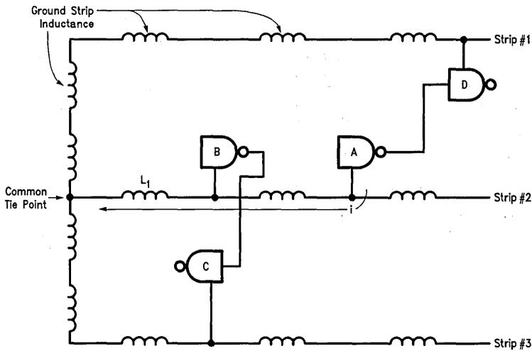
FIGURE 3-19. Ground Trace Coupling
