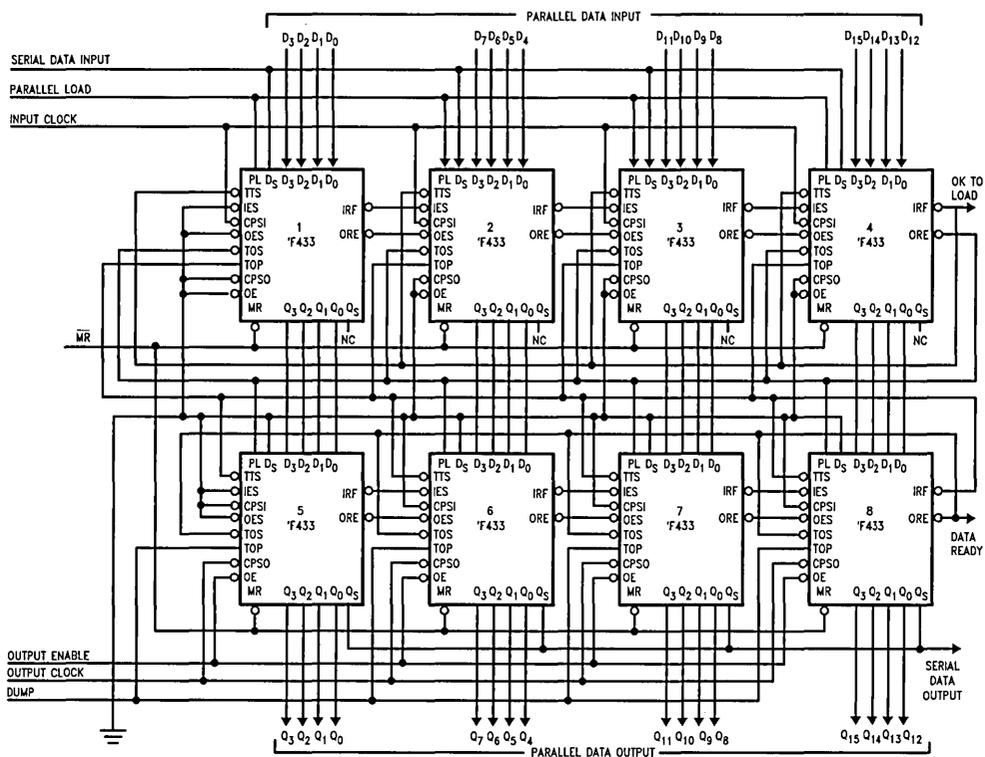
FIGURE 6. A 127 x 16 FIFO Array
