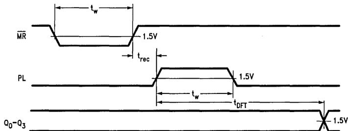
Conditions:  $\overline{TTS}$  connected to  $\overline{TRF}$ ,  $\overline{TOS}$  connected to  $\overline{ORE}$ ,  $\overline{IES}$ ,  $\overline{OES}$ ,  $\overline{OE}$ ,  $\overline{CPSO}$  LOW, TOP HIGH
