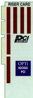
PCI Riser with Three Masters
