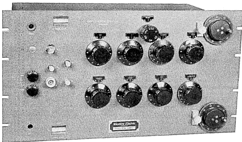
Fig. 6—Front view of the general-purpose bridge shown in Fig. 5. The bridge is approximately 10\frac{1}{2} inches high and 19 inches wide.
