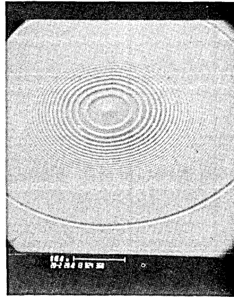
Fig. 2—Scanning electron photomicrographs of etched fiber cross sections illustrate dopant concentration profiles for a boron graded profile and a germania graded profile.
