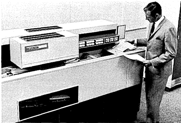
CONTROL DATA 915 Optical Reader . . . "sees" your printed and typewritten material. Inputs data directly, without need for converting it to punched cards, tape, or other intermediate formats.
