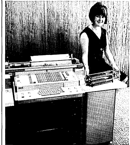
— NCR 395-300. Conventional mechanical "counter line" units, like that held by Gerry Fox, are replaced by magnetic disc memory. Memory of 395 is about the size of a 45 RPM phonograph record.
