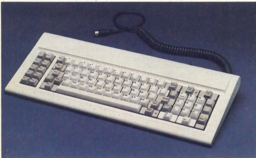
Figure 2: The PC-84D from Hi-Tek uses the Dvorak key layout, with often-used keys in convenient positions. Note that vowels are on the left side of the home row.
