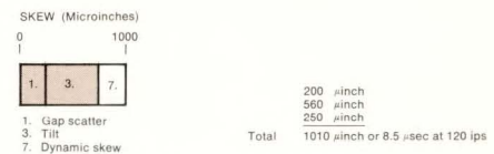
FIGURE 2. Worst case skew for an in-line head assembly. Although it eliminates the major source of errors (stack-to-stack tolerances and dynamics) an in-line head has two drawbacks: 1) crosstalk increases beyond an acceptable level, 2) narrow (non-standard) track spacing is required, which reduces the signal-to-noise ratio, and makes the tape non-interchangeable. Recording all time-related data in the same staggered head stack is a commonly used alternative.
