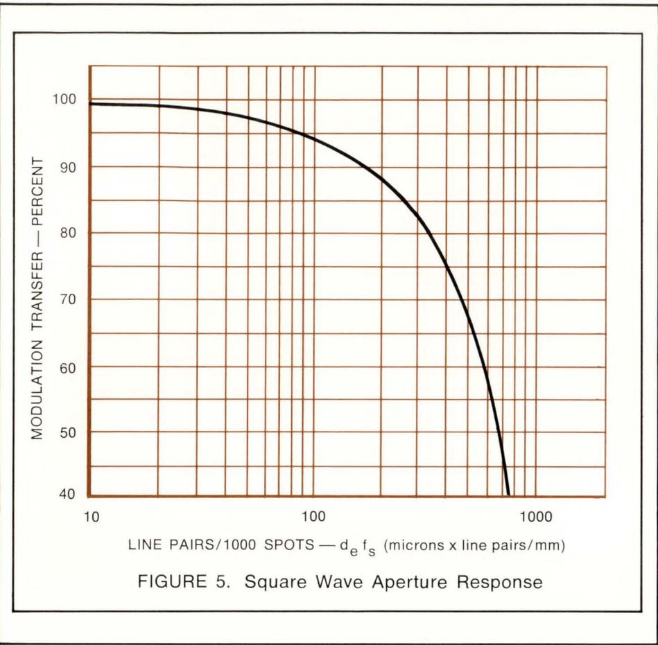
enable beam deflections through 3 to 5 spot diameters to be made at megahertz rates. In the film travel direction, however, deflections of perhaps 30 to 50 spot diameters at much lower bandwidth are required to maintain synchronization between the transport servo and scan line position. This can be obtained by electro-mechanical means. A combination of the two is indicated.
