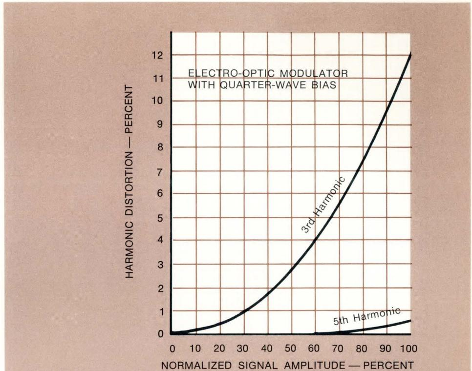
FIGURE 3. Distortion for Biased Electro-optical Modulation
