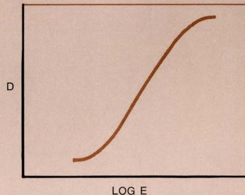
FIGURE 4. Film Transfer Characteristic D-Log E Curve
