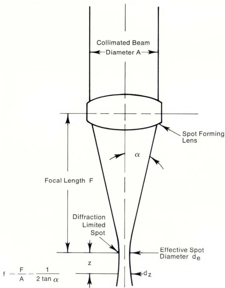
FIGURE 2. Spot Forming Schematic
