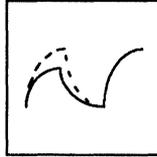
You modify the shape of an object by replacing the closest matching piece of a single object. You use the **Curve Replace** tool to replace part of an object with curved lines.
