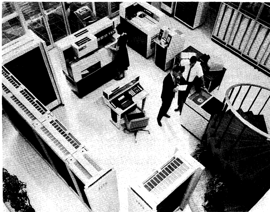
This business-oriented Control Data 3500 configuration features the 915 Page Reader (at left rear).
