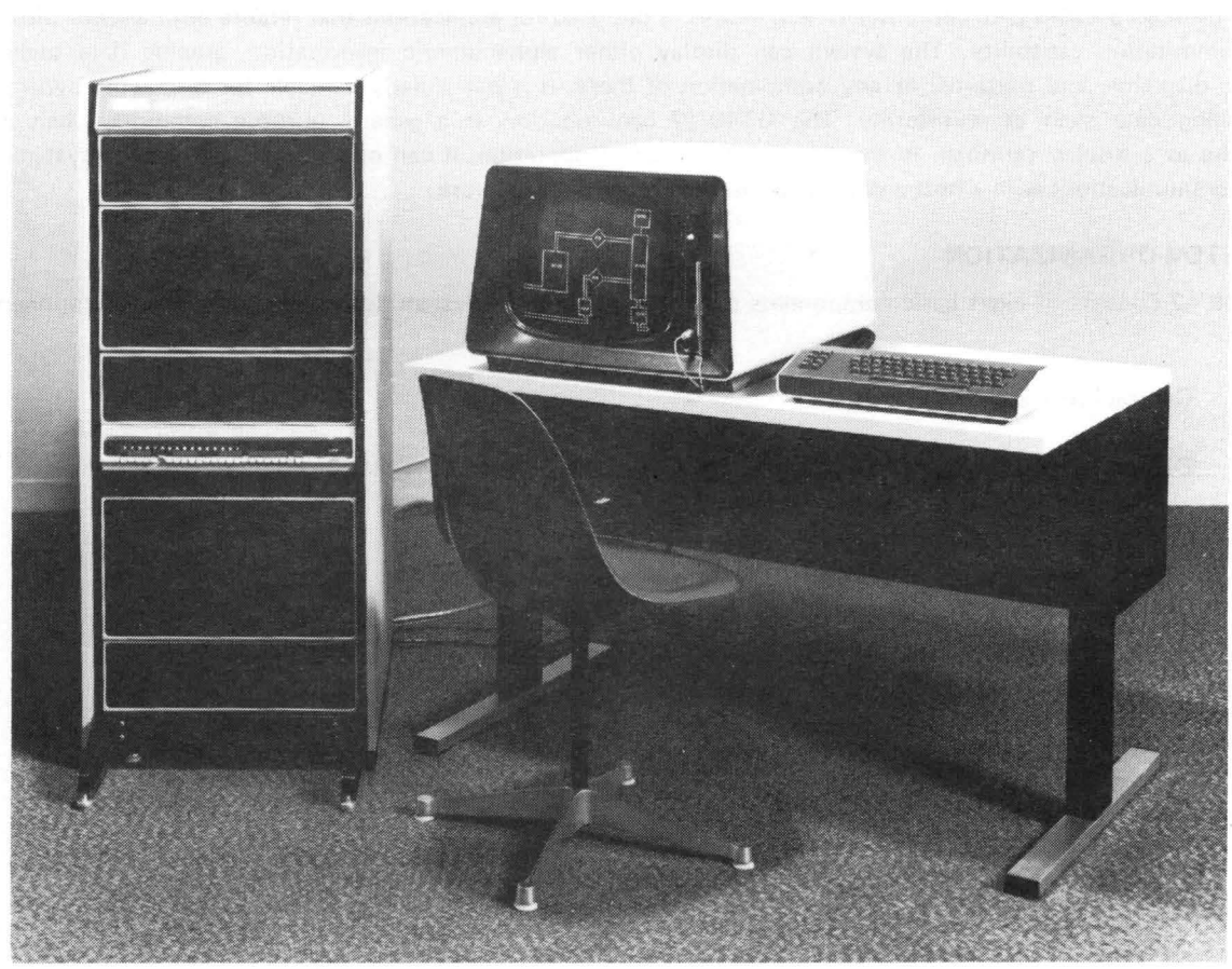
Figure 2 GT42 Graphic Display Terminal
