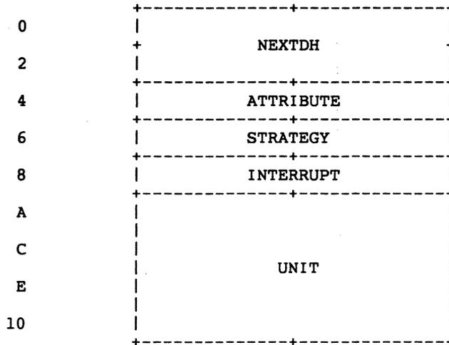
Figure 9-1. DOS Device Header
