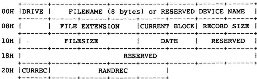
Figure 7-2. DOS Standard File Control Block
