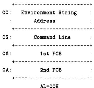
**Figure 7-7. EXEC Load and Execute Parameter Block**
