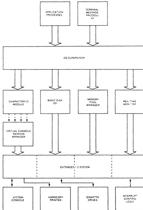
Figure 1-1. Concurrent DOS 86 Virtual/Physical Environments
