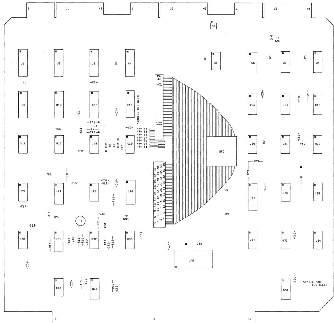
Figure 8-3. Model 64151A Component Locator (64151-66503)
