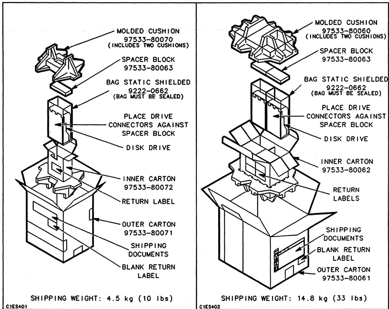
Figure 2-1. Single-Unit Packaging Kit, HP 19518A
