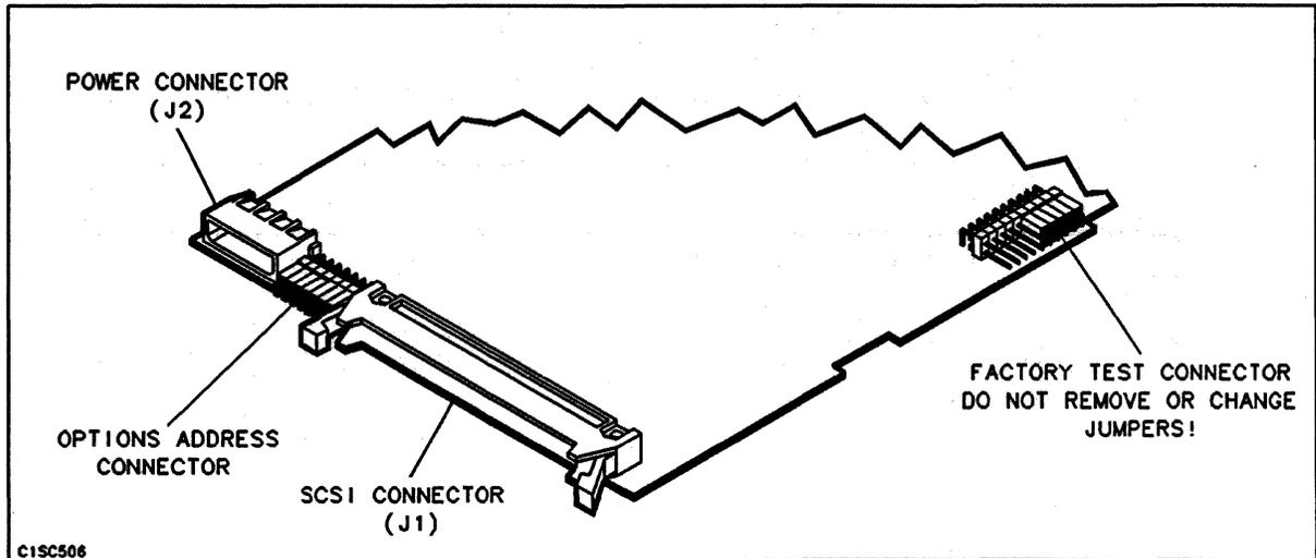
Figure 3-6. Factory Test Connector Location
