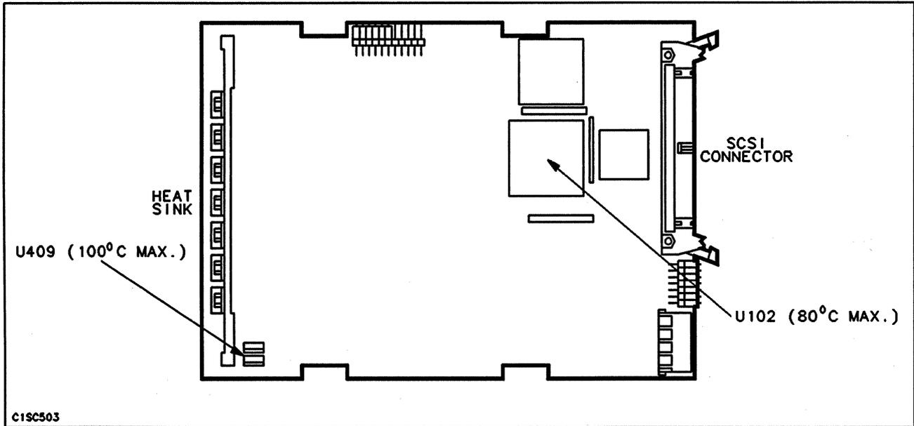
Figure 3-3. PCA Temperature Measuring Points
