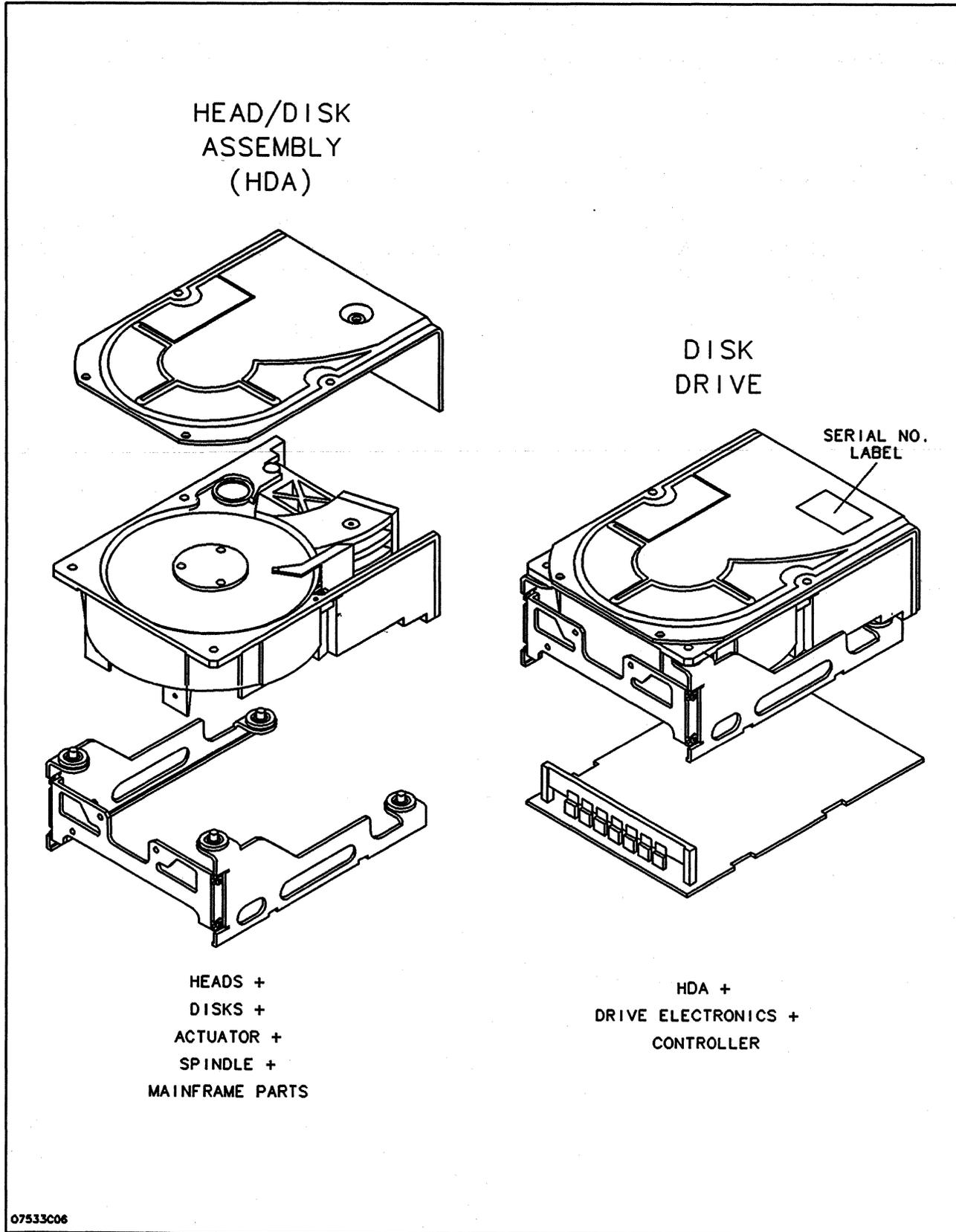
Figure 1-1. Disk Mechanism Major Components
