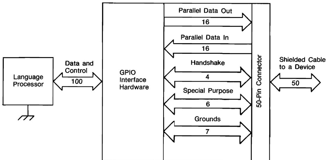
Three lines are dedicated to handshaking the data from source to destination device. The Peripheral Control line (PCTL) is controlled by the interface and is used to initiate data transfers. The Peripheral Flag line (PFLG) is controlled by the peripheral device and is used to signal the peripheral's readiness to continue the transfer process. The Input/Output line (I/O) is used to indicate direction of data flow.
