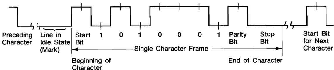
**Parity.** The parity bit is used to detect errors as incoming characters are received. If the parity bit does not match the expected sense, the character is assumed to be incorrectly received. The action taken when an error is detected depends upon how the interface and your computer program are configured.
