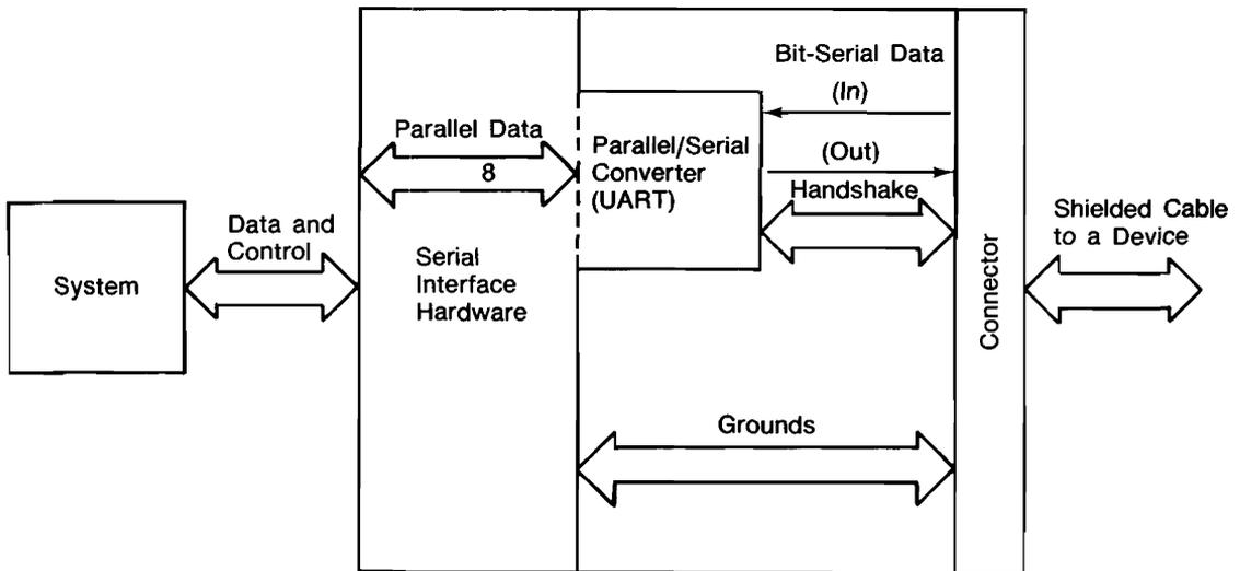
The RS-232-C interface standard establishes electrical and mechanical interface requirements, but does not define the exact function of all the signals that are used by various manufacturers of data communications equipment and serial I/O devices. Consequently, when you plug your serial interface into an RS-232 connector, there is no guarantee the devices can communicate unless you have configured optional parameters to match the requirements of the device you are connecting to.
