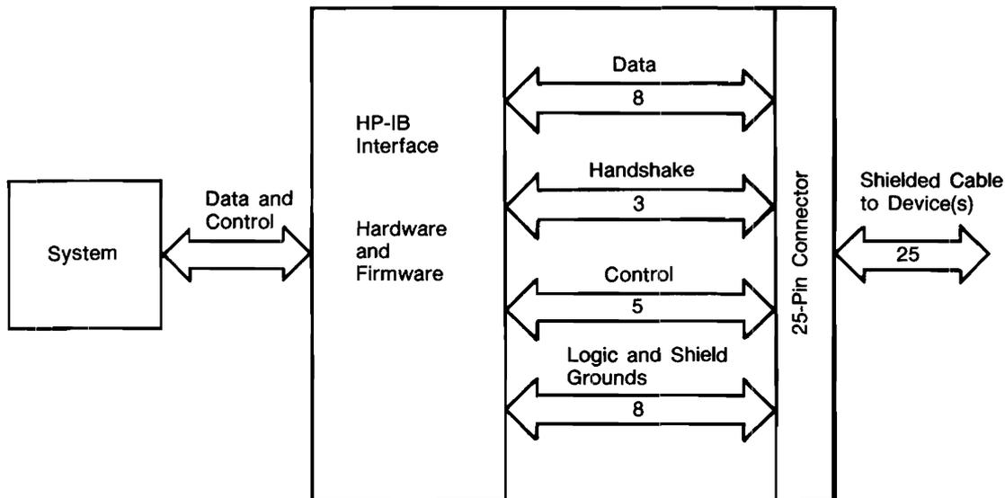
The HP-IB Interface is easy to use and allows great flexibility in communicating data and control information between the computer and external devices.
