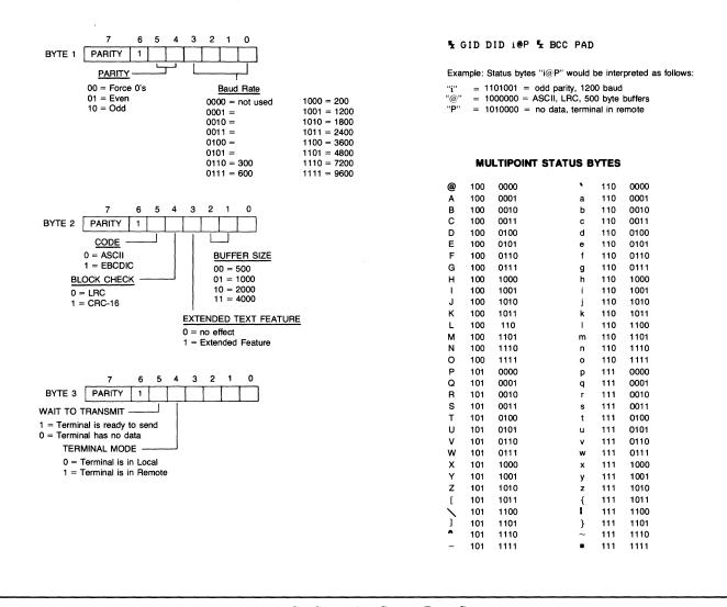
Figure 5-16. Configuration Status Byte Contents
