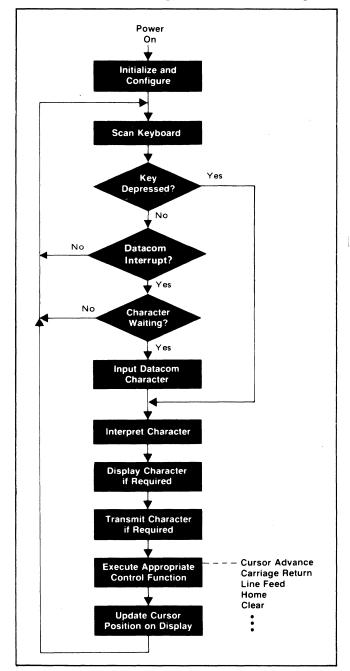
Figure 1-3. System Monitor Basic Loop
