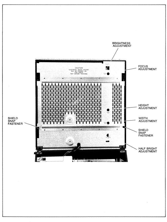
Figure 7-3. Mainframe Top Part Locations
