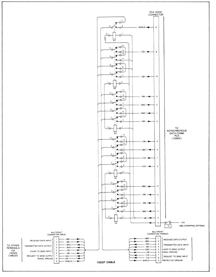
Figure 7-24. Power-Down-Protect Cabling for Asynchronous Multipoint Configuration
