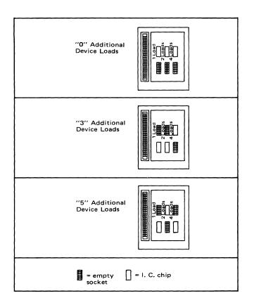
Figure 8-3. Selecting Additional Device Loads
