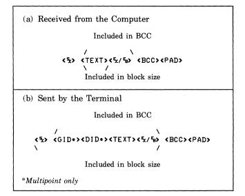
Figure 5-11. Examples of Block Transmission
