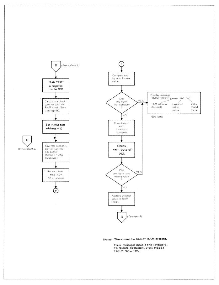
Figure 7-30. Basic Terminal Self-Test Flowchart (Sheet 2 of 3)
