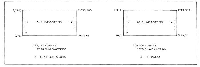
Figure 3-25. Comparison of a Terminal with 1024  $\times$  780 Display and the HP 2647A
