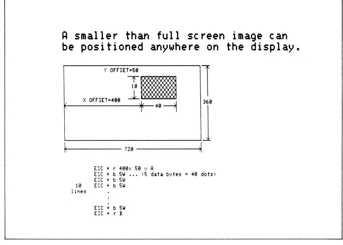
Figure 3-12. Raster Data Positioning
