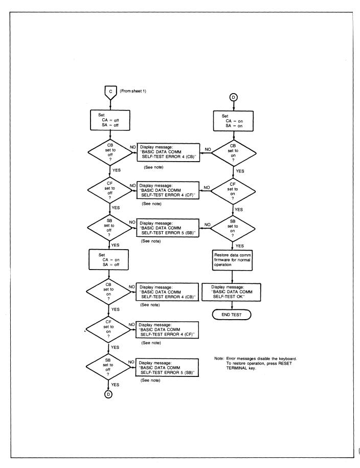
Figure 7-31. Basic Data Comm Self-Test Flowchart (Sheet 2 of 2)
