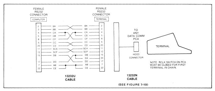
Figure 7-21. Modem By-Pass Cabling
