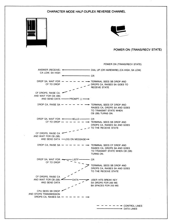
Figure 5-9. Sample Data Transfers Using Reverse Channel Protocol
