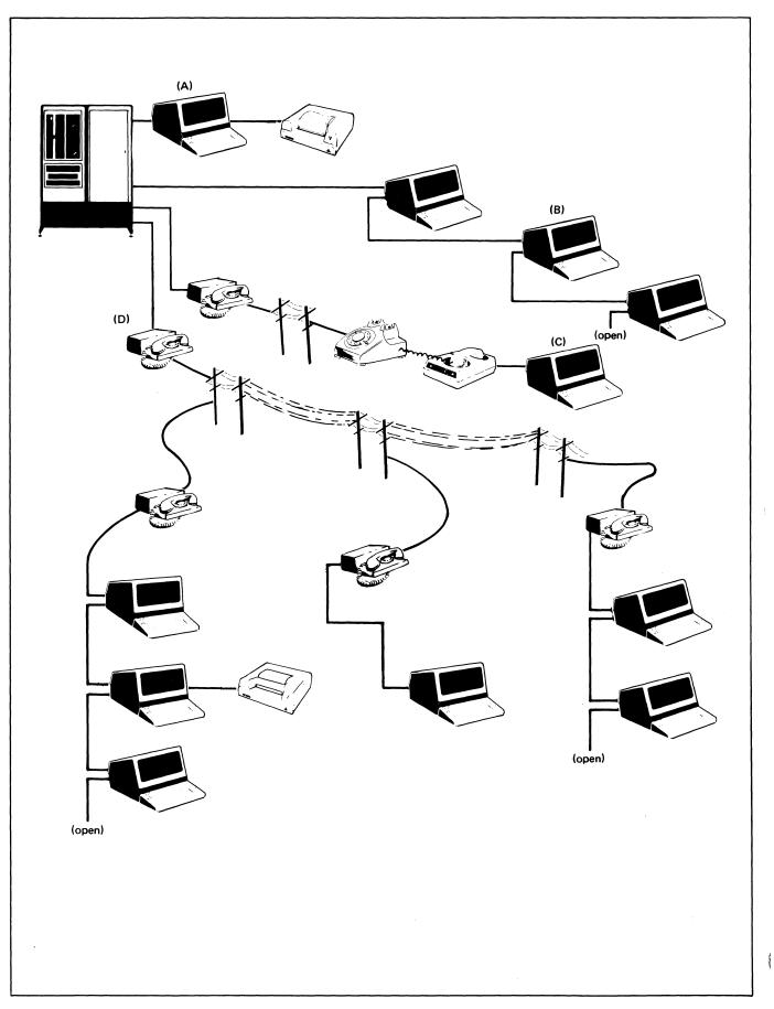
Figure 5-1. Terminal Network Configurations
