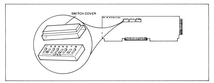
Figure 7-14. Typical Strapping Option Switch Assembly
