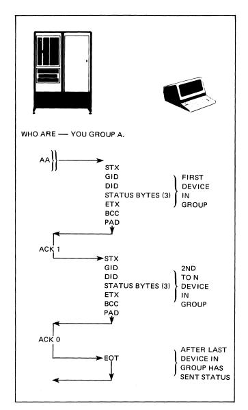
Figure 5-15. Typical Configuration Status Request and Response Sequence
