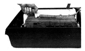
Figure 7-7. Top Plane Assembly Removal
