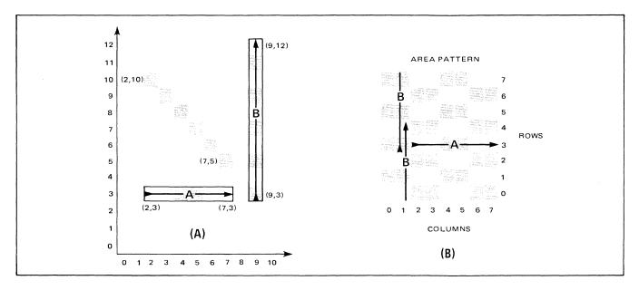
Figure 3-4. Using Area Patterns As Line Types
