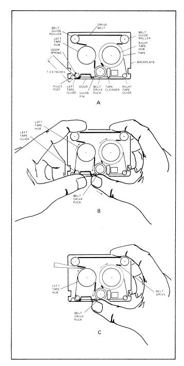
Figure D-1. Tape Cartridge Rethreading
