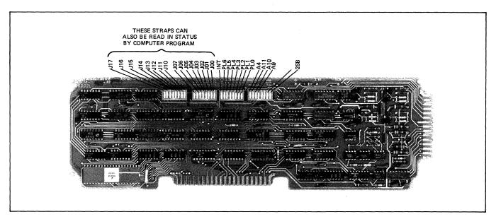
Figure 7-17. Asynchronous Multipoint Communications PCA Strapping Options
