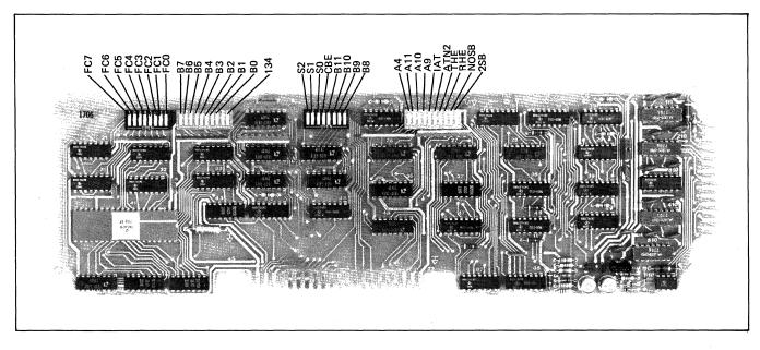
Figure 7-16. Extended Asynchronous Communications PCA Strapping Options
