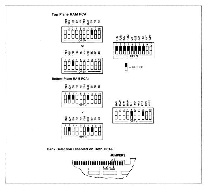
Figure 7-8. 32K RAM PCA Jumper Settings
