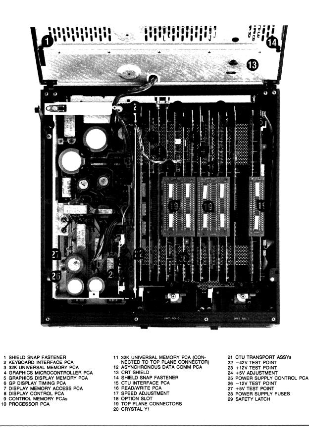
Figure 7-2. Mainframe Bottom Part Locations
