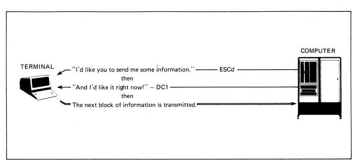
Figure 5-3. Block Transfer Enabled By The Computer
