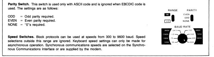
Figure 5-13. Block Keyboard Data Communication Switches
