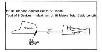
As you can see from the above examples, should you need extra cable length at some point within your configuration you can obtain it by simulating extra device "loads" with the HP-IB Interface Adapter. Your configuration is, however, always limited to a combined total of 20 meters of interconnecting cable or a total of 15 devices (actual plus simulated).
