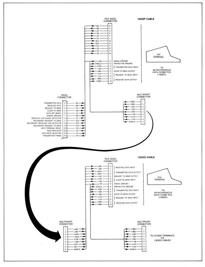
Figure 7-22. Asynchronous Multipoint Cabling
