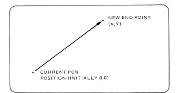
Figure 3-8. Current Pen Position And New End Point
