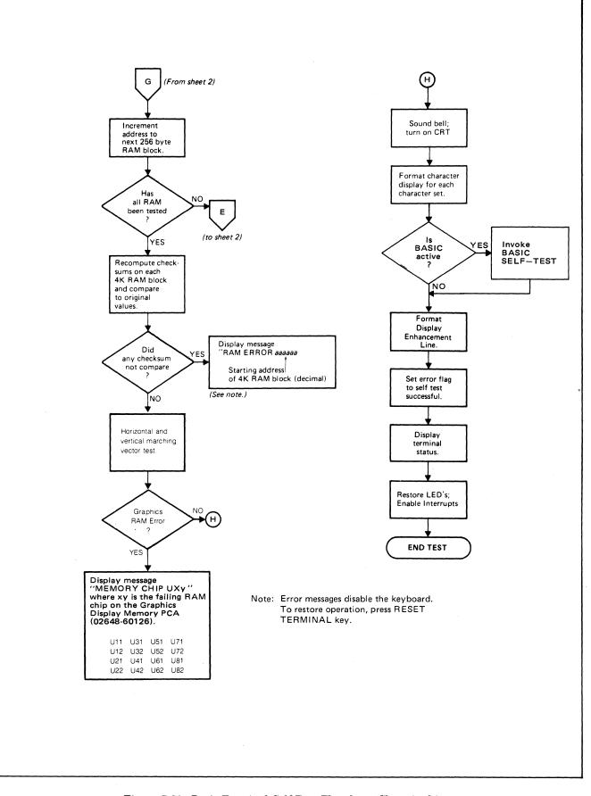
Figure 7-30. Basic Terminal Self-Test Flowchart (Sheet 3 of 3)
