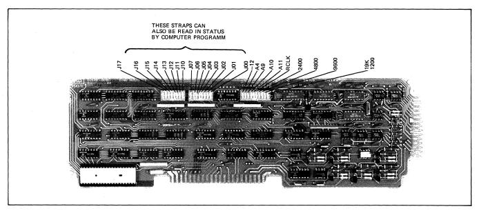
Figure 7-18. Synchronous Multipoint Communications PCA Strapping Options
