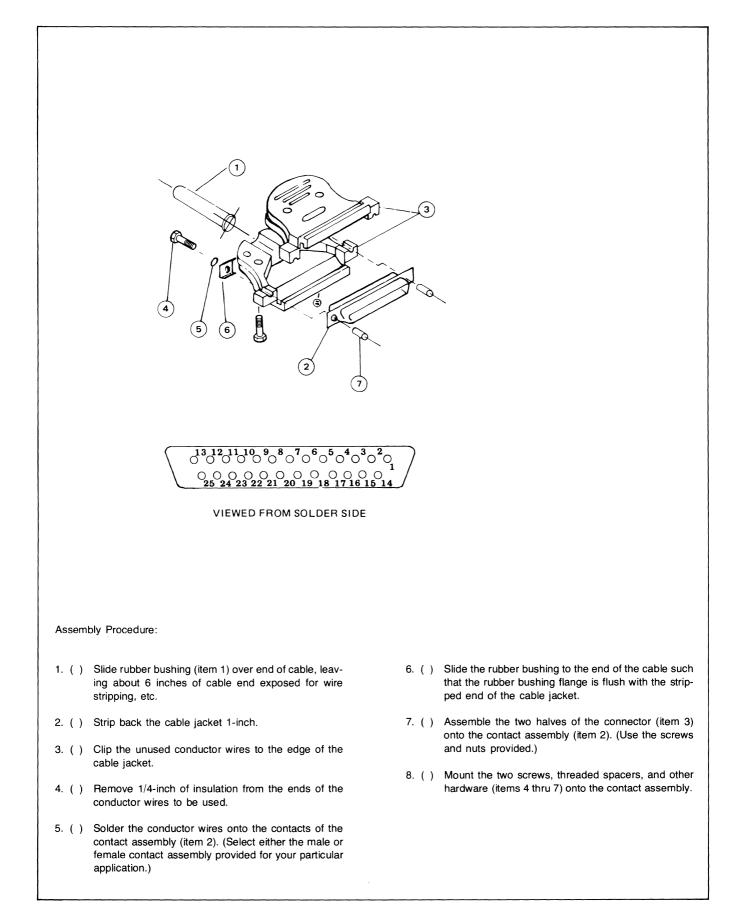
Figure 7-27. Assembling the RS232C Connector
