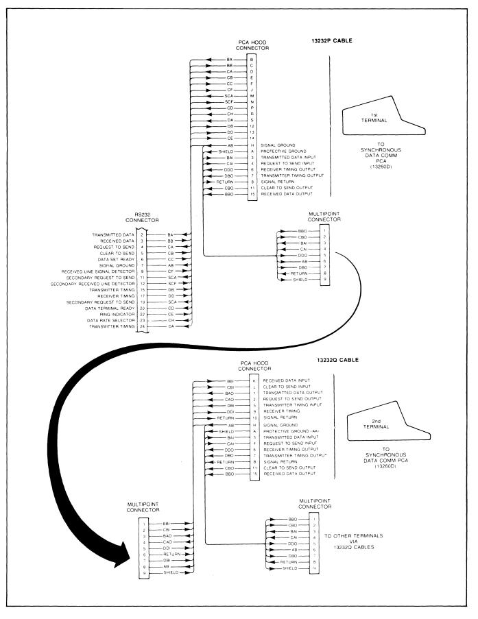
Figure 7-23. Synchronous Multipoint Cabling
