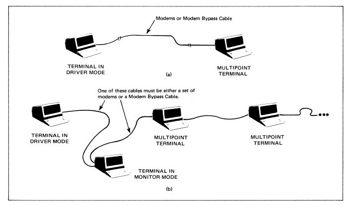
Figure 5-22. Driver Mode Configurations
