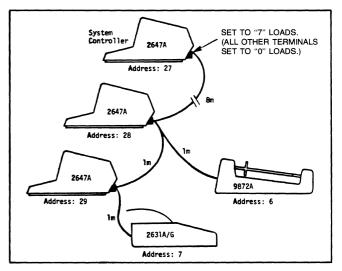
Figure 8-6. 3-Terminal, Shared Plotter/Printer Configuration
