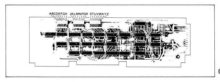
Figure 7-15. Keyboard Interface PCA Strapping Options
