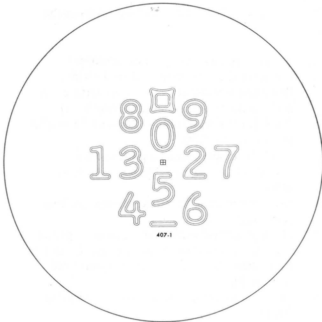
Figure A-8. 407-1 Reticle for Pocket Comparator
