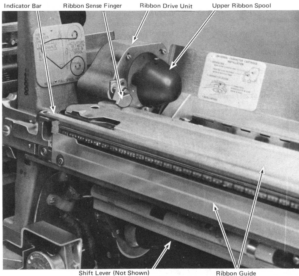
Figure 4-54. Ribbon Drive Assembly
