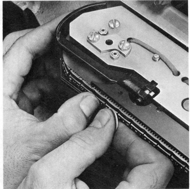
Figure 4-44. Method of Separating Type Slugs
