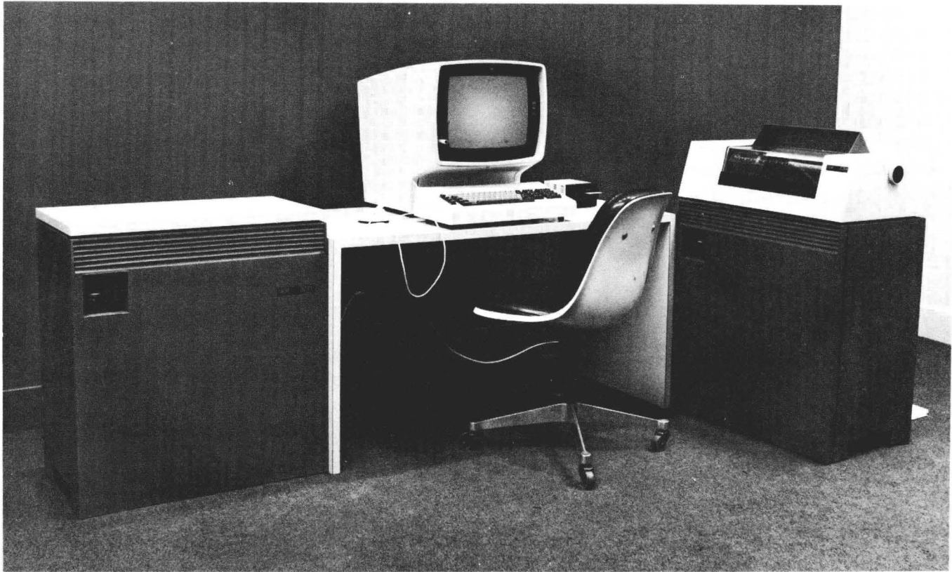
Frontispiece. IBM 3270 Information Display System: 3271/3272 Control Unit, and Attached 3277 Display Station and 3284/3286 Printer
