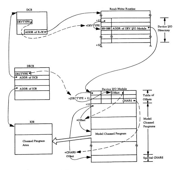
Figure 26. Read-Write pointers and tables
