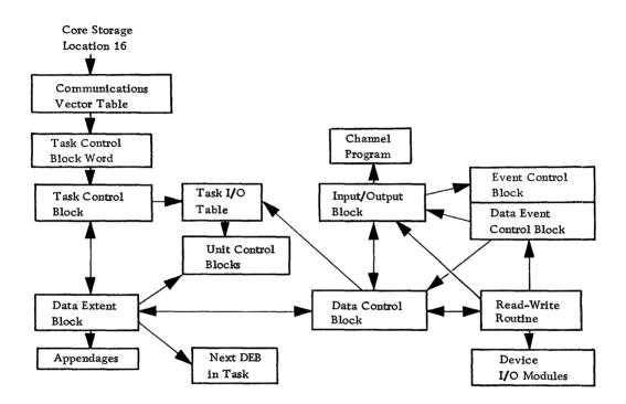
Figure 15. OS/360 control block linkages
