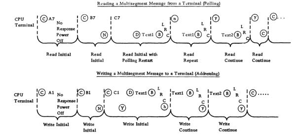
Figure 2. Examples of IBM 1050 line control
