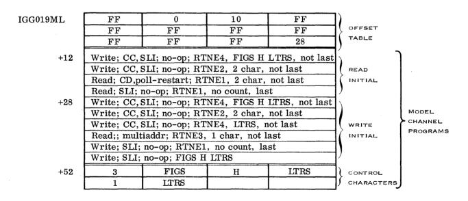
Figure 13. Device I/O Module for AT&T 83B3
