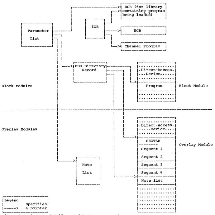
Figure 9. Blocks and Tables Used by Program Fetch
