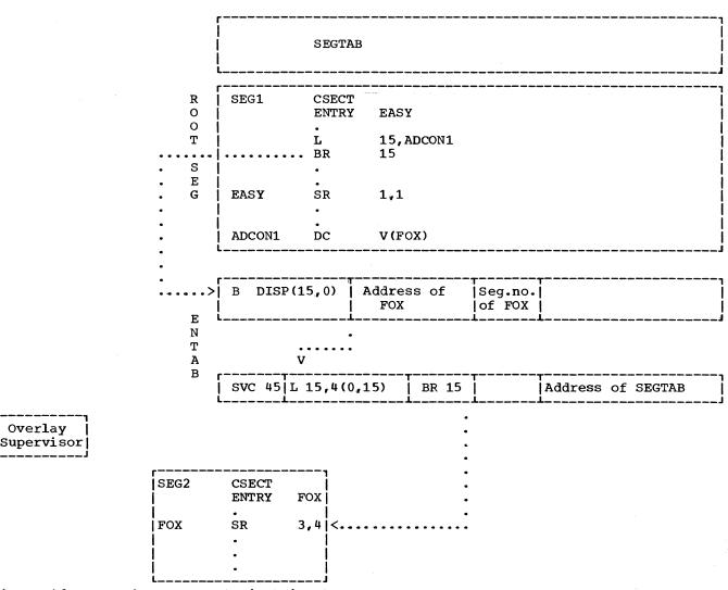
Figure 16. Branch to Segment in Main Storage
