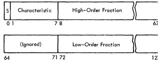
Figure 2-10. Extended Floating-Point Number Format
