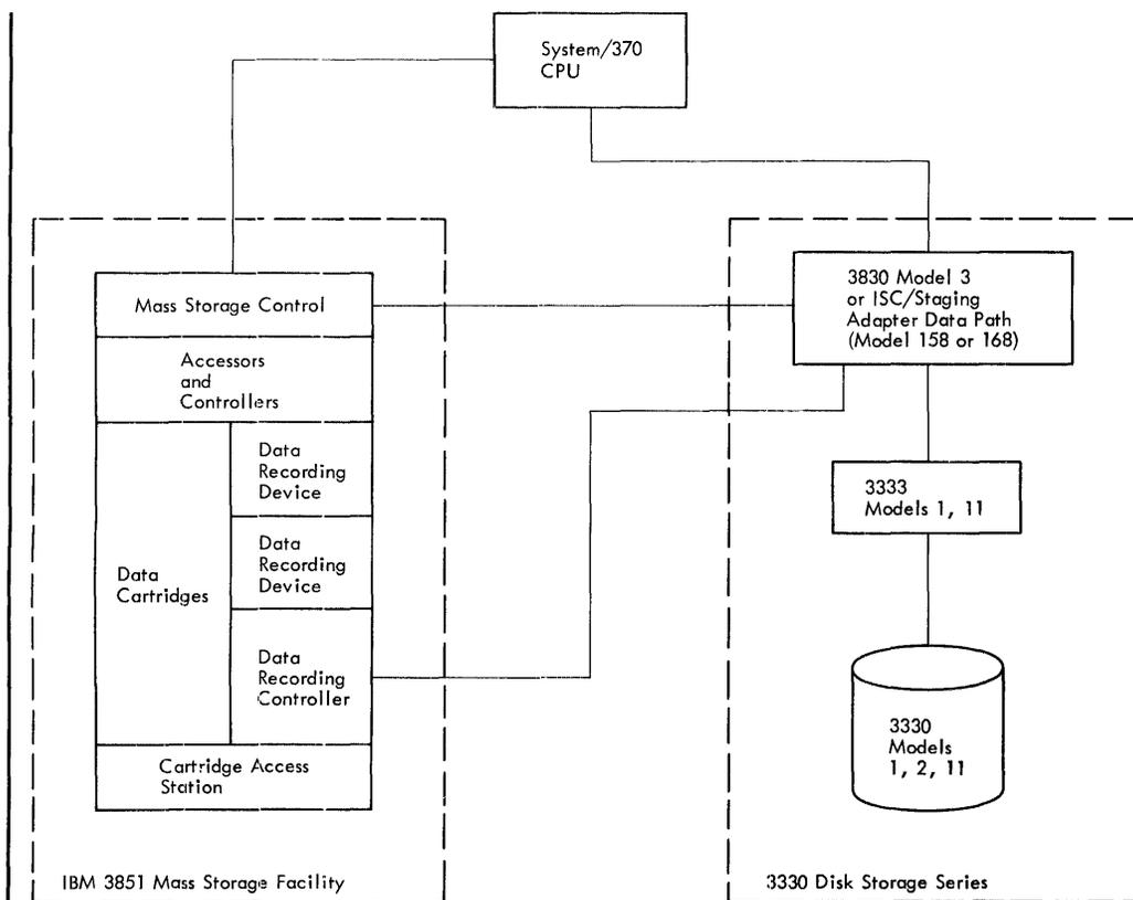
Figure 7-72. Logical Components of IBM 3850 Mass Storage System
