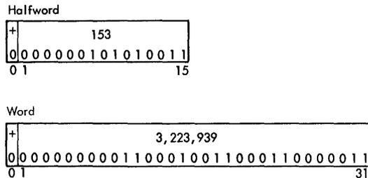
Figure 2-7. Fixed-Point Number Formats (with Signed Binary Data)
