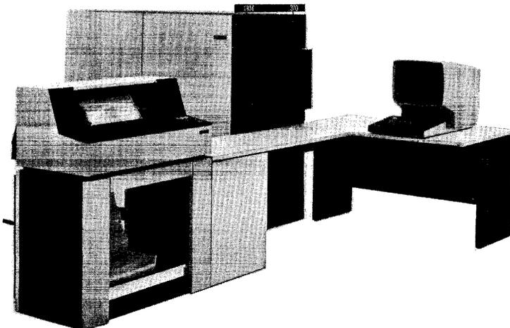
Figure 6-1. IBM System/370 Model 115 with IBM 3203 Printer
