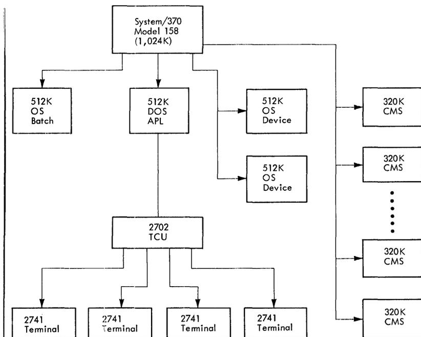
Figure 4-8. Virtual Machines for Concurrent Program Maintenance
