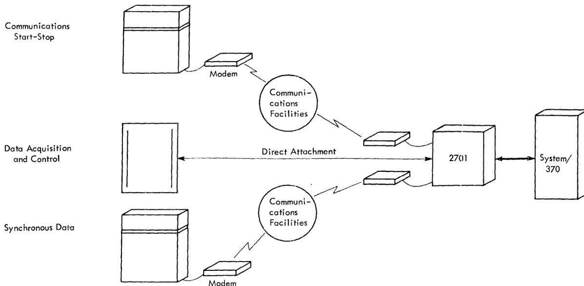
Figure 8-3. An IBM 2701 in a System Environment
