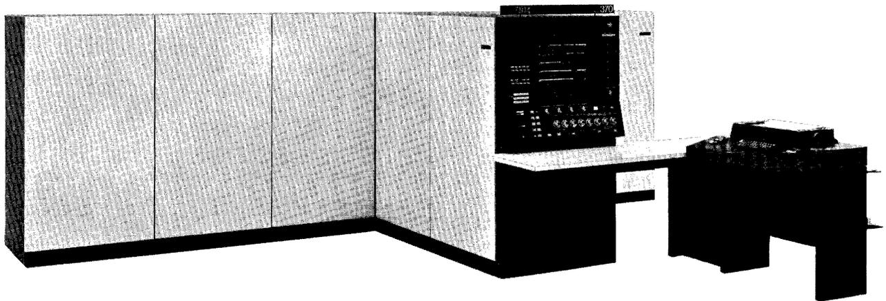
Figure 6-5. IBM System/370 Model 155 with IBM 3210 Console Printer-KeyBoard
