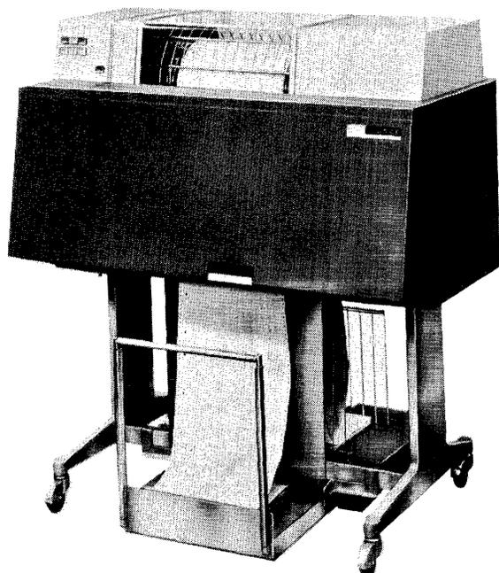
Figure 7-48. IBM 1403 Printer Models 2, 3, and 7
