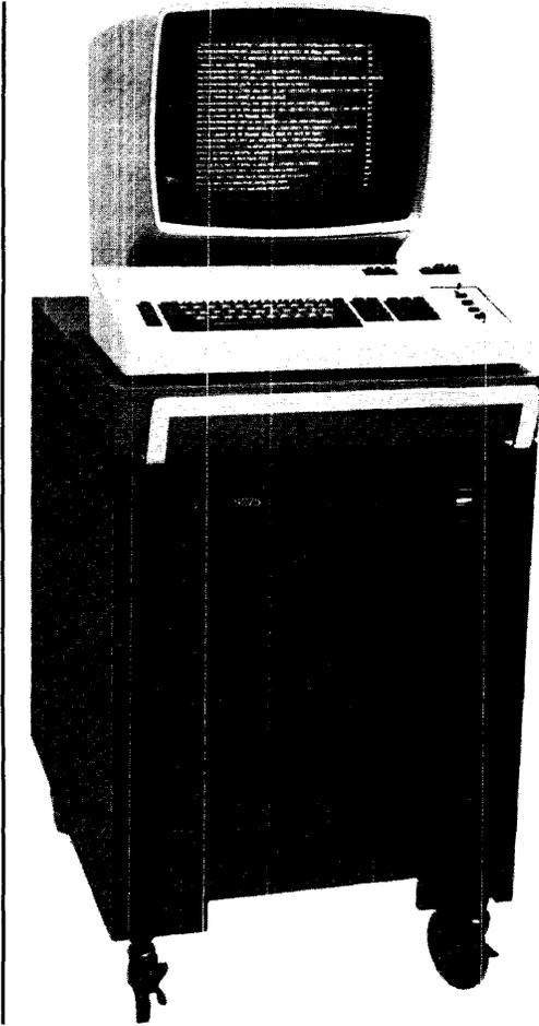
Figure 8-19. IBM 5275 Direct Numerical Control Station
