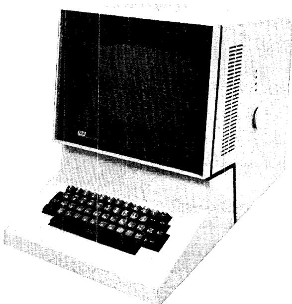
Figure 7-21. IBM 2260 Display Station with an Alphanumeric Keyboard
