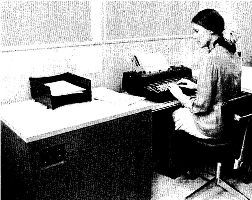
Figure 8-16. IBM 3735 Programmable Buffered Terminal
