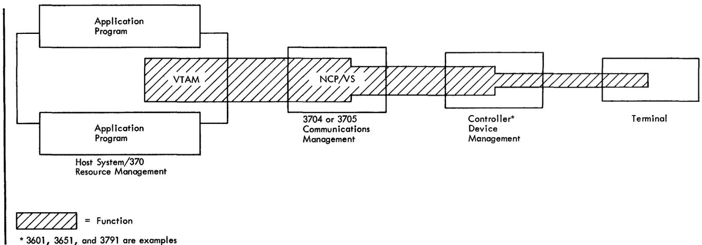
Figure 5-5. Concept of Function Distribution under Programming Control
