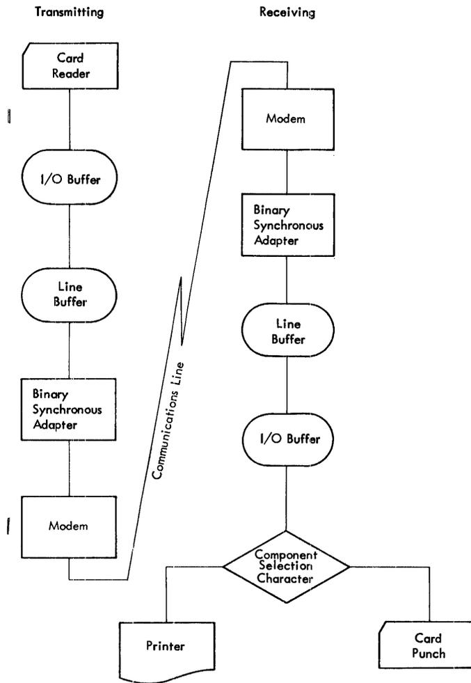
Figure 8-14. Data Flow, Terminal-to-Terminal Operation
