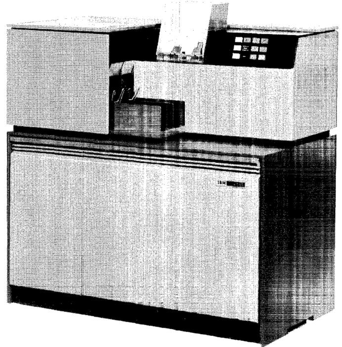
Figure 7-57. IBM 2520 Card Read Punch Model B1
