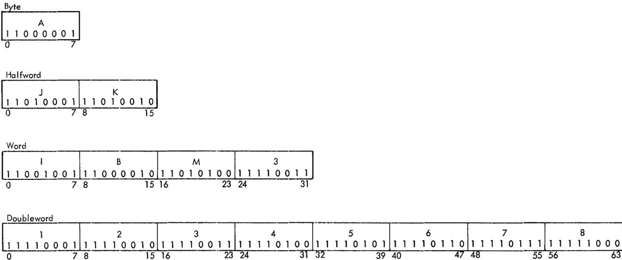
Figure 2-2. Basic Fixed-Length Data Formats (with EBCDIC-Coded Data)
