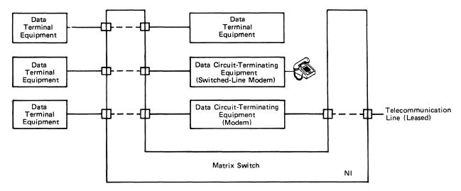
Figure 1-2. Matrix Switch in a Telecommunication Network
