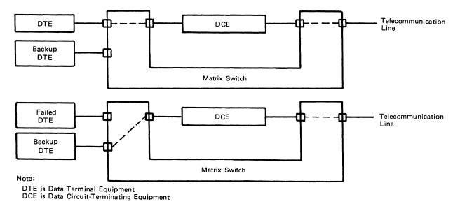
Figure 2-2. Sparing a Failed DTE
