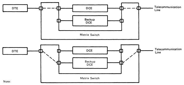
DTE is Data Terminal Equipment DCE is Data Circuit-Terminating Equipment
