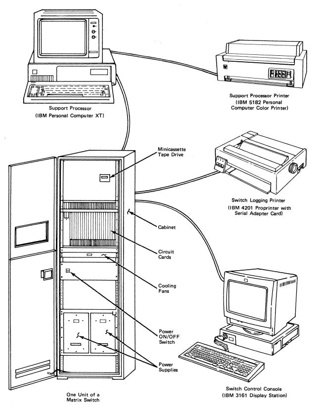
Figure 3-1. Major Components of a Matrix Switch
