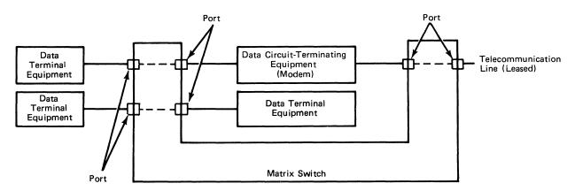
Figure 2-1. Matrix Switch Port Connections
