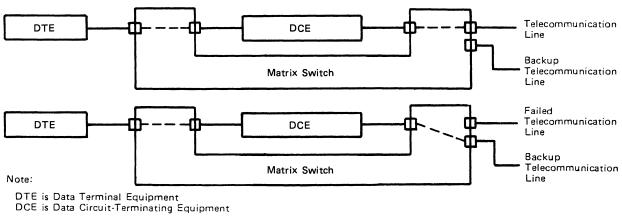
Figure 2-4. Sparing a Failed Telecommunication Line
