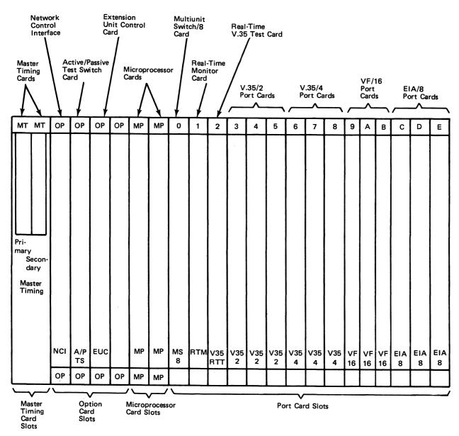
Figure 3-2. Matrix Switch Card Cage
