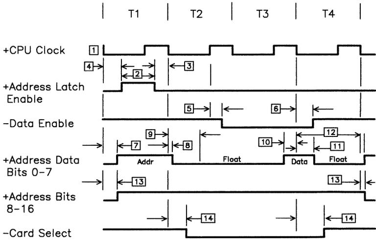
**Figure C-7 (Part 2 of 2). Memory Interface, Processor Read**
