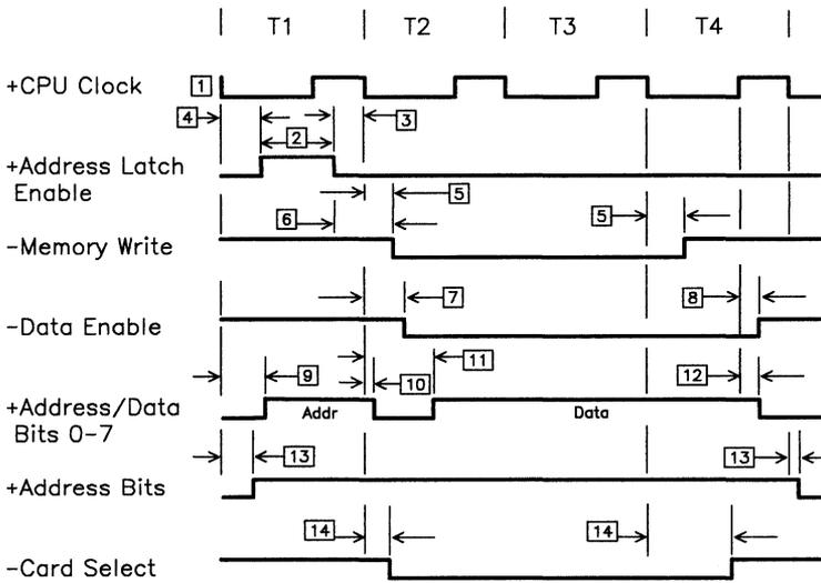
**Figure C-8 (Part 2 of 2). Memory Interface, Processor Write**
