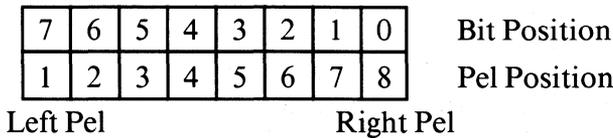
**Figure 2-18. High Resolution Bit-to-Pel Relationship**
