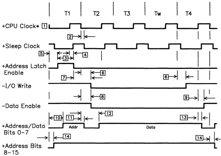
**Figure C-6 (Part 2 of 2). I/O Interface, Processor I/O Write**
