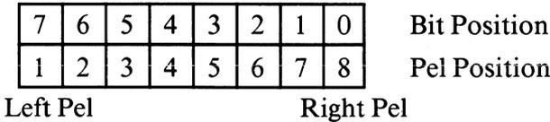
**Figure 3-11. High Resolution Bit-to-Pel Relationship**
