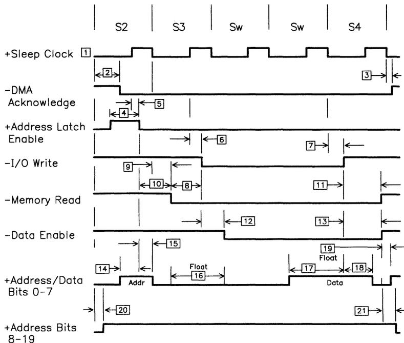
**Figure C-3 (Part 2 of 2). I/O Interface, DMA from Memory to I/O**
