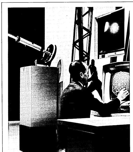
BEAMS OF INFRARED LIGHT are carrying high-speed messages in two experimental applications at Canada's Expo 67. In one application, a light beam transmits stock-market quotations from the 19th floor of the Montreal Stock Exchange to closed-circuit television units in the Canadian Government Pavilion—a distance of almost two miles. Another beam travels a half mile from the IBM Computer Room in the Canadian Government Pavilion to a 2250 Display Unit in the Man the Producer Pavilion. The technique, developed by IBM engineers, involves the conversion of electronic signals to variations in the intensity of infrared light, which is invisible. In the photograph above, retouching depicts a light beam entering the receiving unit. The data carried by the beam is reconverted to electrical impulses for display on the 2250 terminal.
