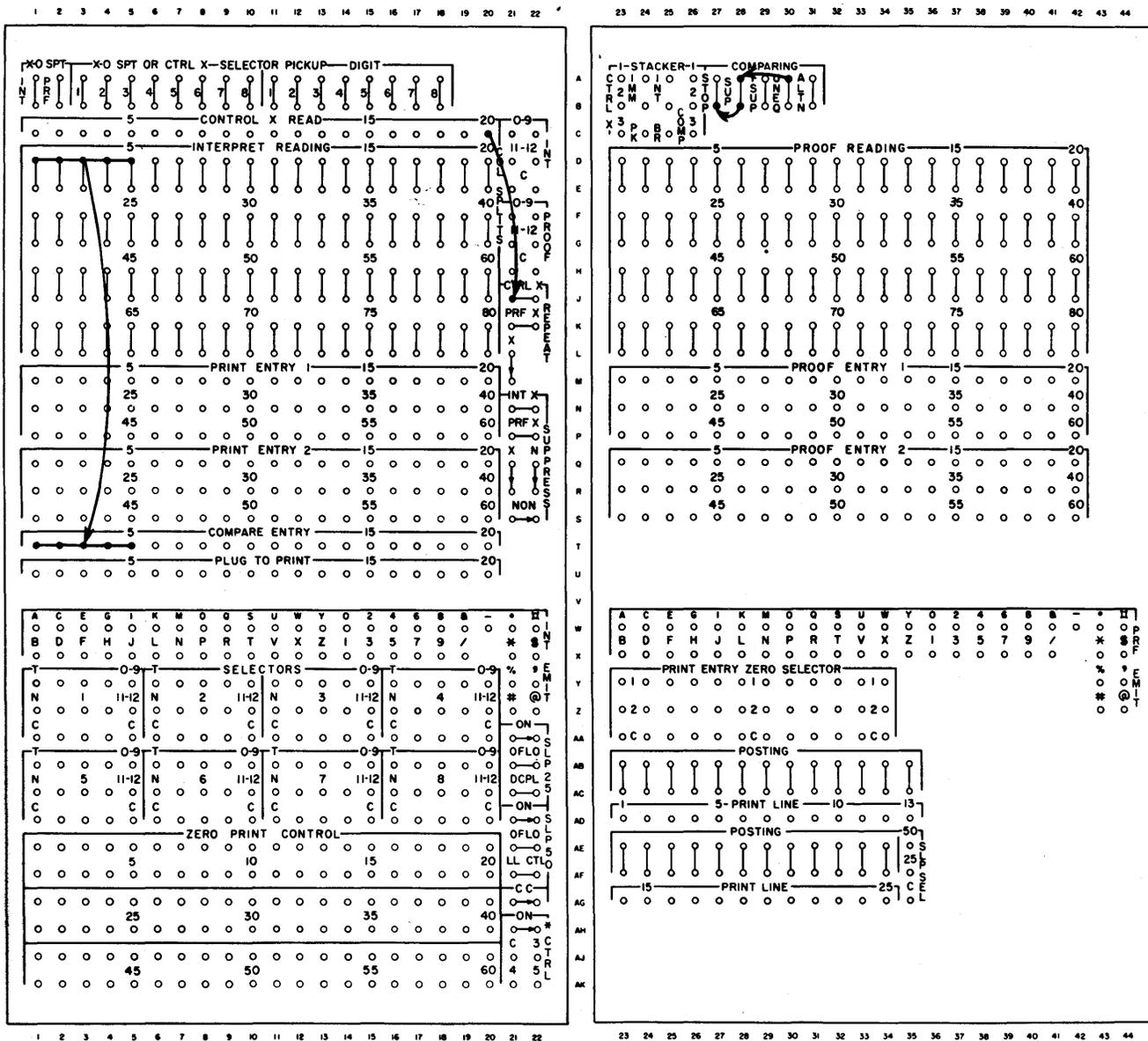
FIGURE 124. IBM 557 CONTROL PANEL WIRED FOR CARD-TO-CARD COMPARING
