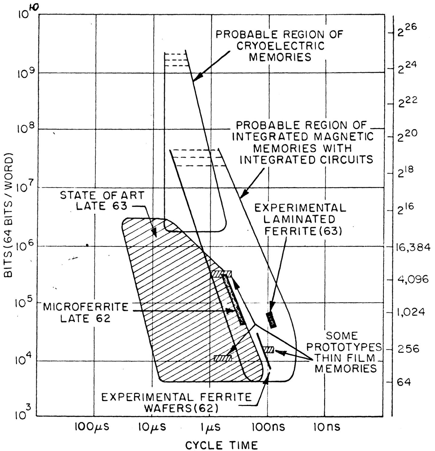
Figure 2-35 - Storage Capacity and Cycle Time of Memories
