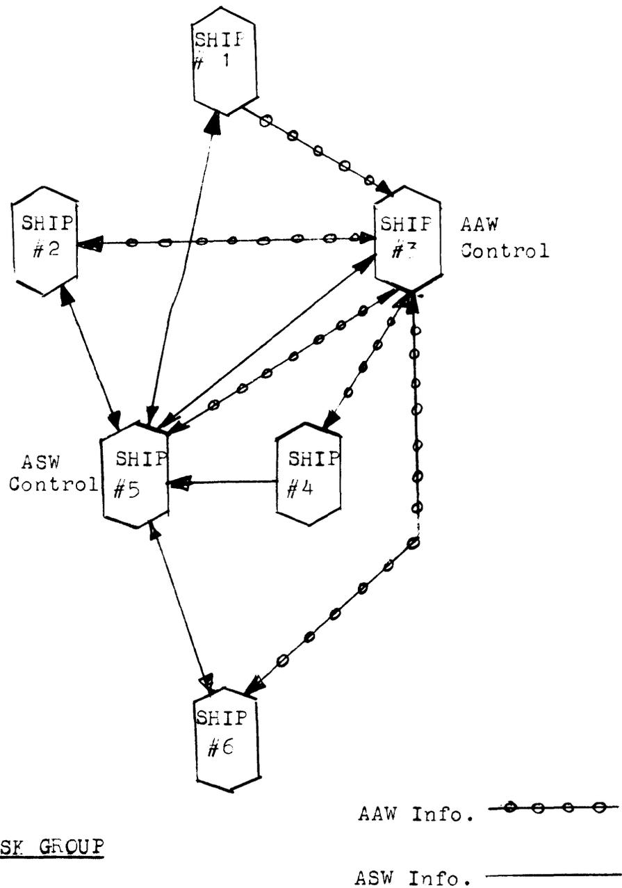
Figure 4-2; CENTRALIZED SYSTEM CONTROL
