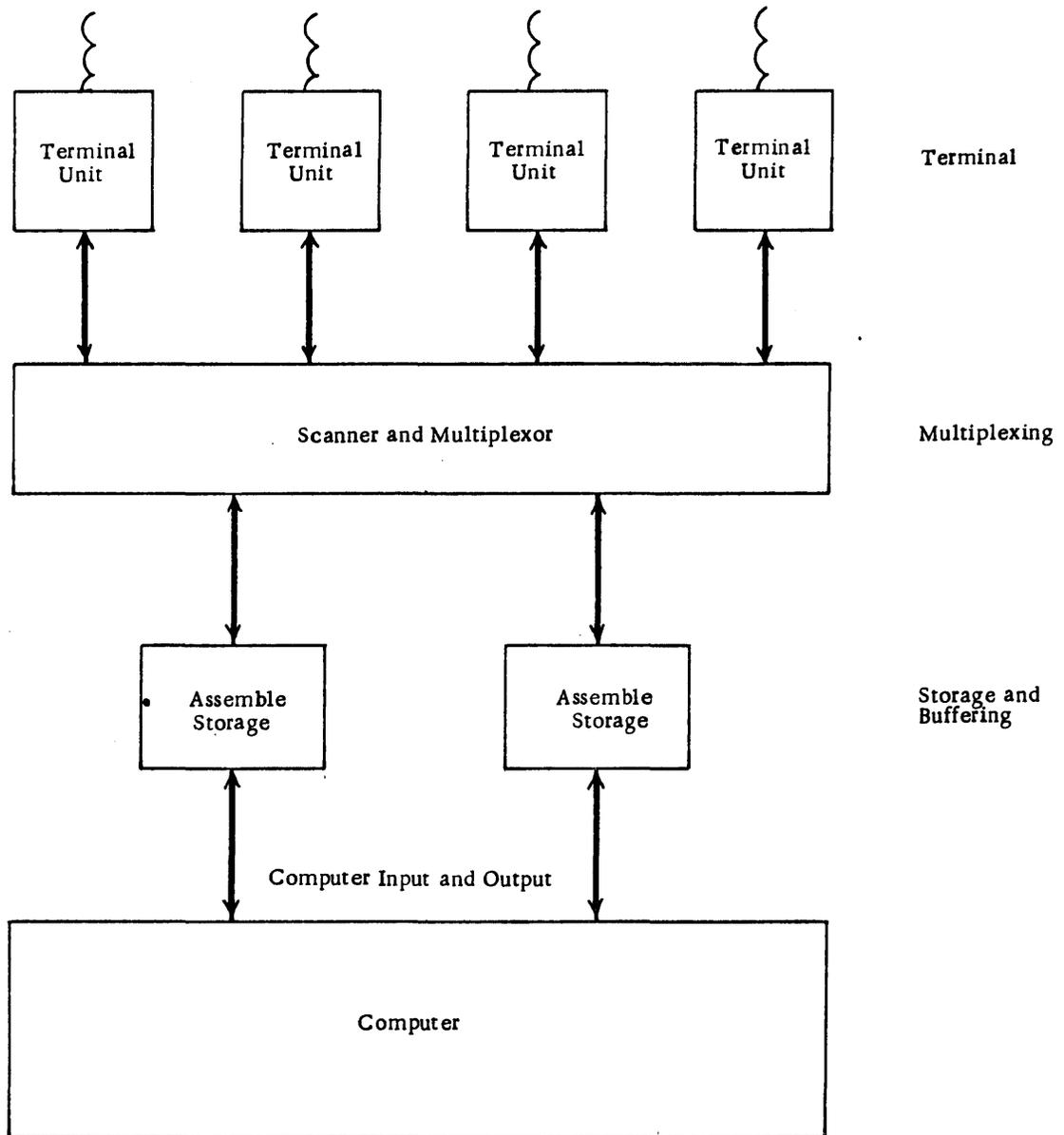
Figure 2-34 Schematic of Typical Interface Functions in Digital Machine-to-Machine Communication
