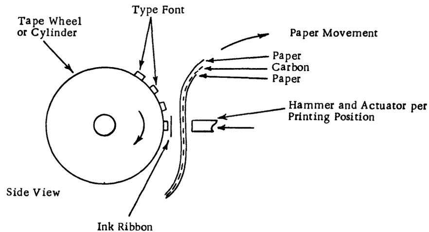
Figure 2-24 Rotating Drum Printer
