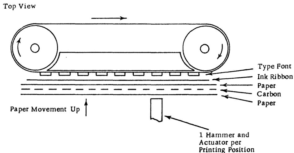
Figure 2-28 Chain Printer
