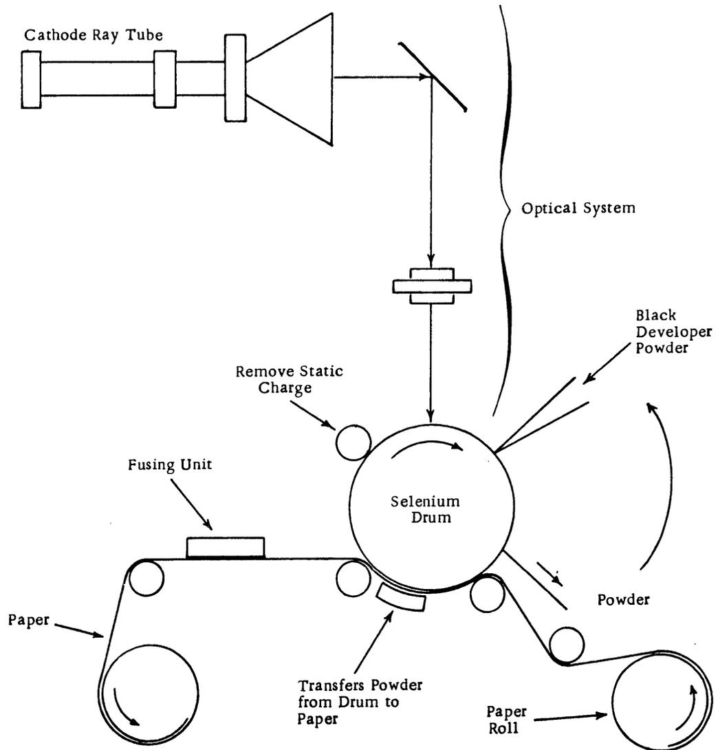
Figure 2-30 Electro-Optical Printer
