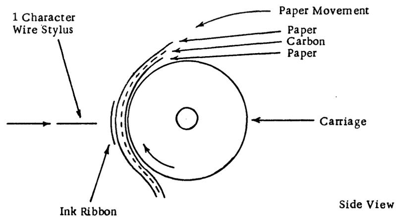
Figure 2-27 Stylus Printer
