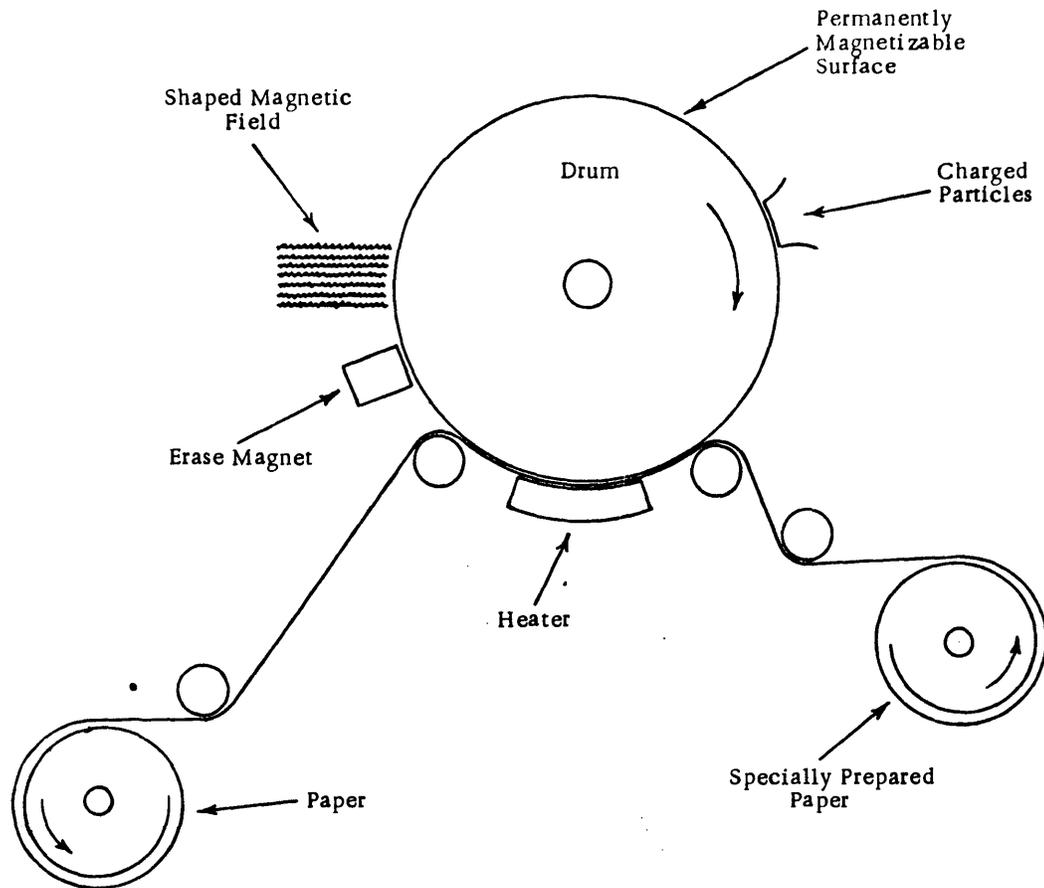
Figure 2-32 Magnetic Printer
