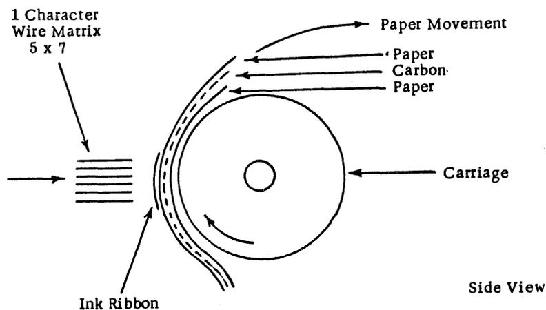
Figure 2-26 Matrix Printer
