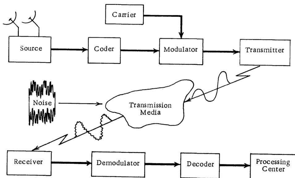
Figure 3-6, Carrier Transmission System
