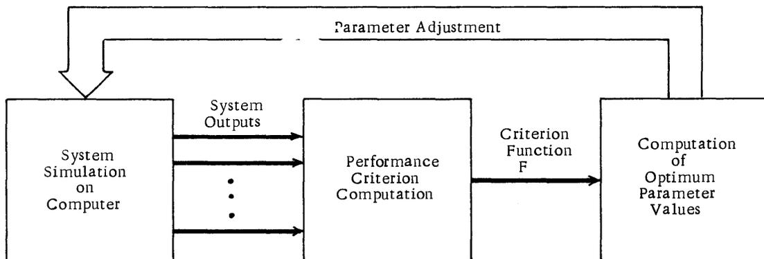
Figure 3-5, Block Diagram of Design Optimization Problem
