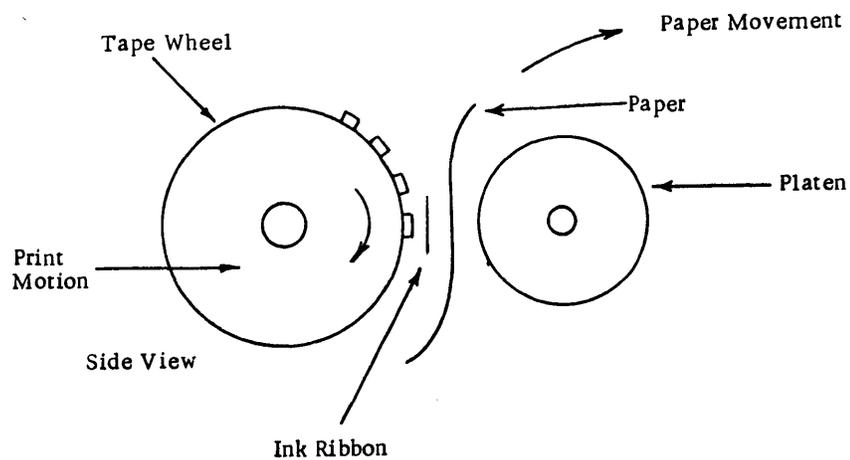
Figure 2-25 Impact Wheel Printer
