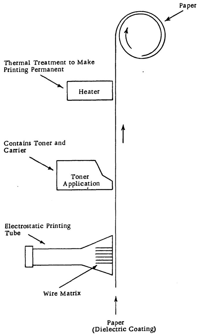
Figure 2-31 Electrographic Printer
