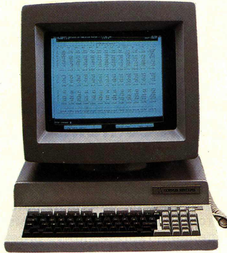
In the horizontal position, the screen can show 48 rows of 120 characters.
