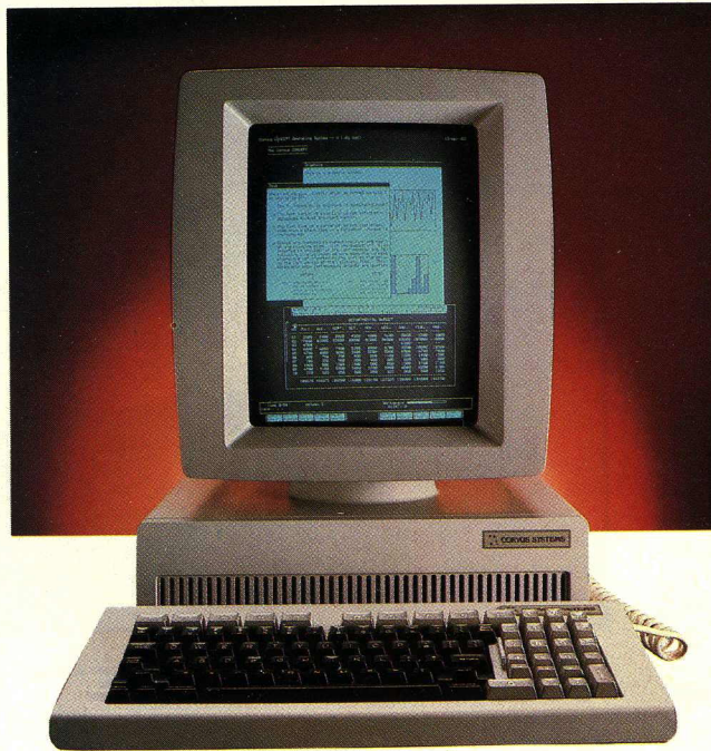
The Personal Workstation's flexible display can accommodate up to 17 sub-screens.
