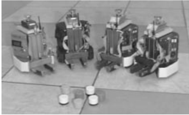
Figure 1-12: The mobile robots used to validate the group behavior and learning methodologies described in this thesis. These robots demonstrated learning to forage by using group safe-wandering, following, and resting behaviors.
