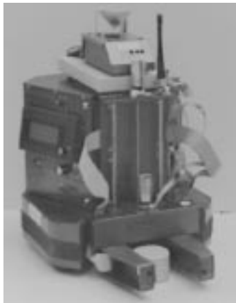
Figure 8-2: Each of the learning robots consists of a differentially steerable wheeled base and a gripper for grasping and lifting objects. The robot's sensory capabilities include piezo-electric bump and gripper sensors, infra-red sensors for collision avoidance, and a radio transmitter for absolute positioning.
