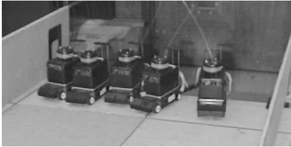
Figure 5-18: The end result of the docking behavior of five robots.
