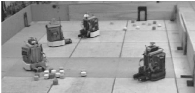
Figure 8-7: A typical environment state during the course of a learning experiment. Since they are learning independently, the robots have likely acquired different parts of the policy. Through interactions with objects in the world and each other they accumulate learning trials in order to complete their learning.
