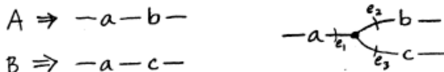
Figure 5.1. Flow grammar fragment and pseudo-flow graph. The graph displays fan-out and can be considered an optimization of the two flow graphs generated by the grammar fragment.
