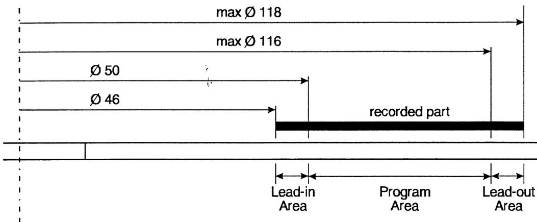
Figure I - 3 Example of the layout of a Finalized disc with one Session
