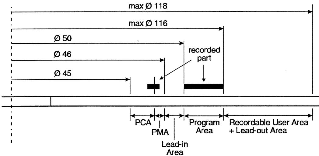
Figure I - 2 Example of the layout of a Partially Recorded disc with one Session
