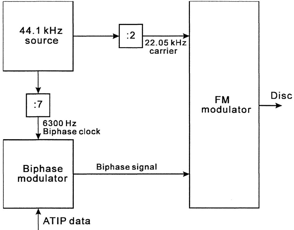
Figure IV - 7.1 Block diagram of a typical ATIP encoder
