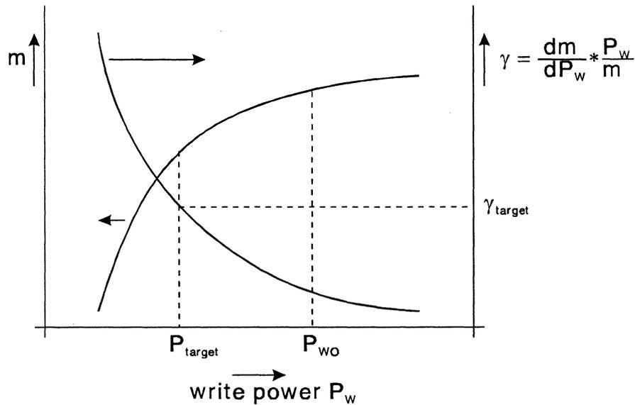
Figure C - 3.1 Modulation and Gamma versus Power function
