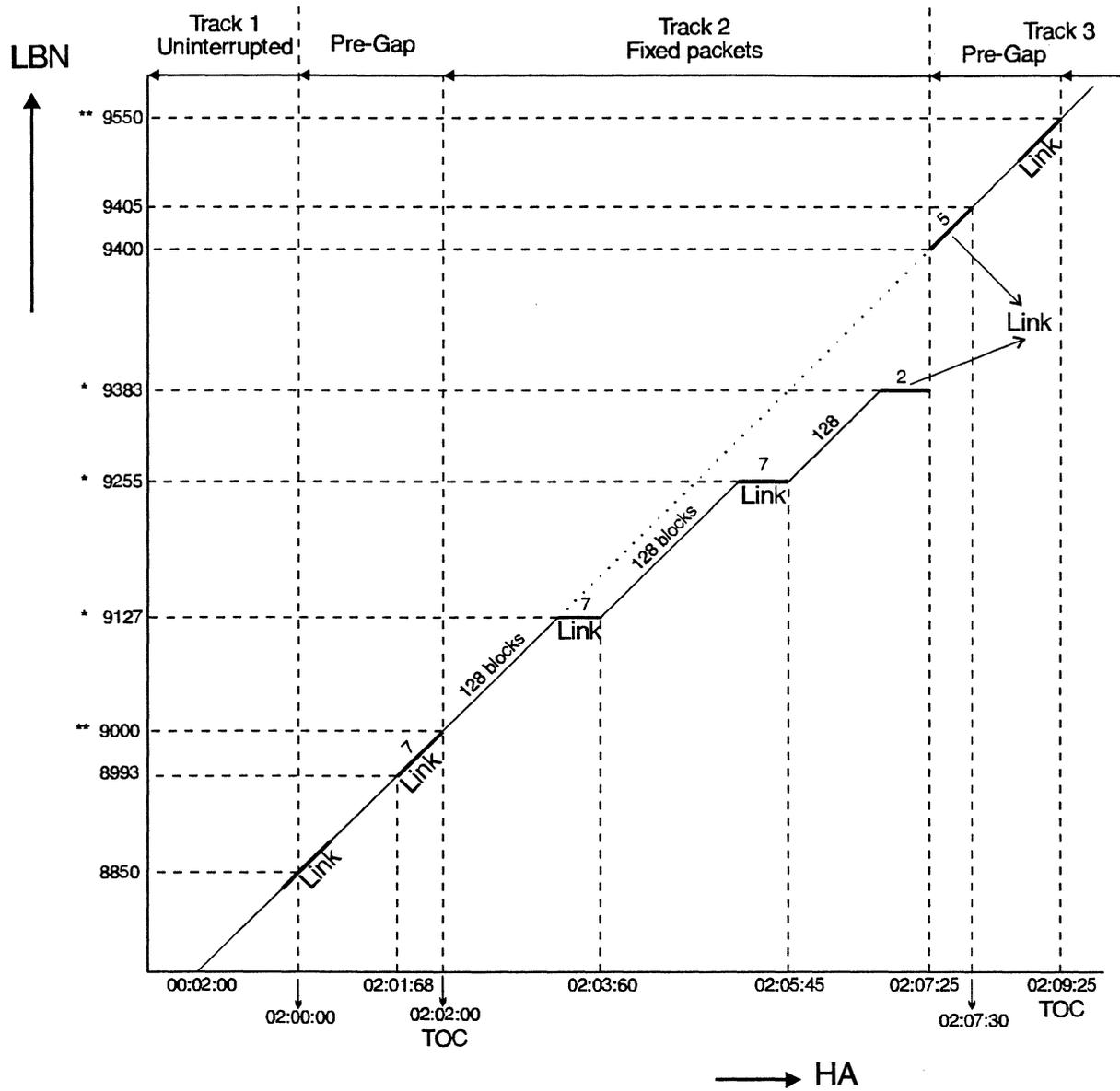
Figure C - 8.1 Example of addressing Method 1 and 2
