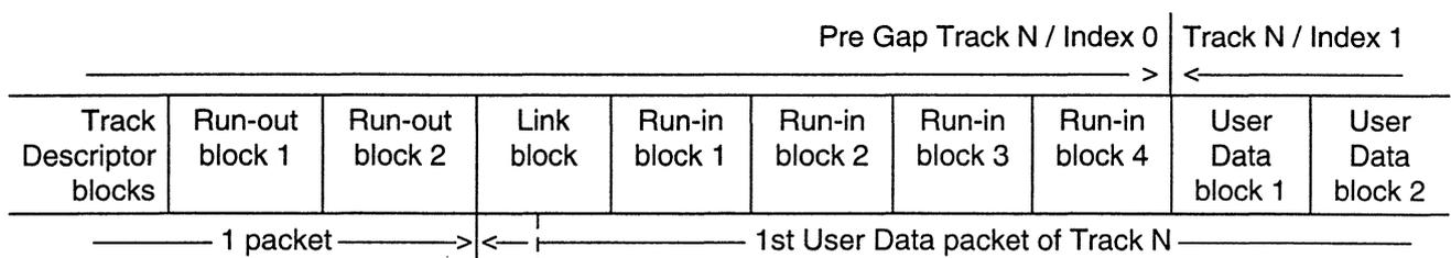
**Figure V - 6.5 Linking of the first User Data in the Track to the Pre Gap**
