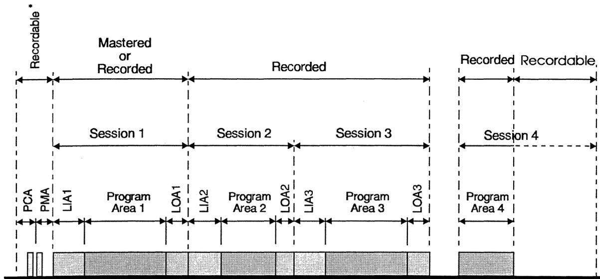
Figure XI - 1 Example of the layout of a Multisession disc
