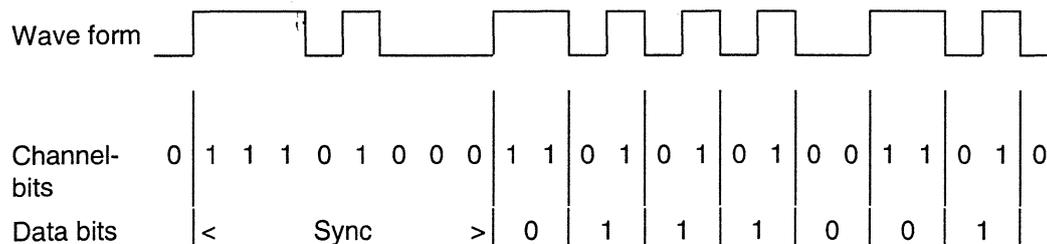
Figure IV - 3.2 Example 1 of the synchronization of the ATIP frames
