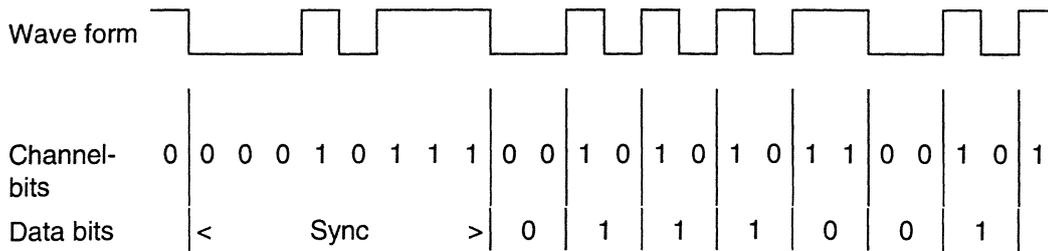
Figure IV - 3.3 Example 2 of the synchronization of the ATIP frames
