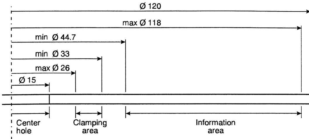
Figure I - 1 Layout of the Unrecorded disc
