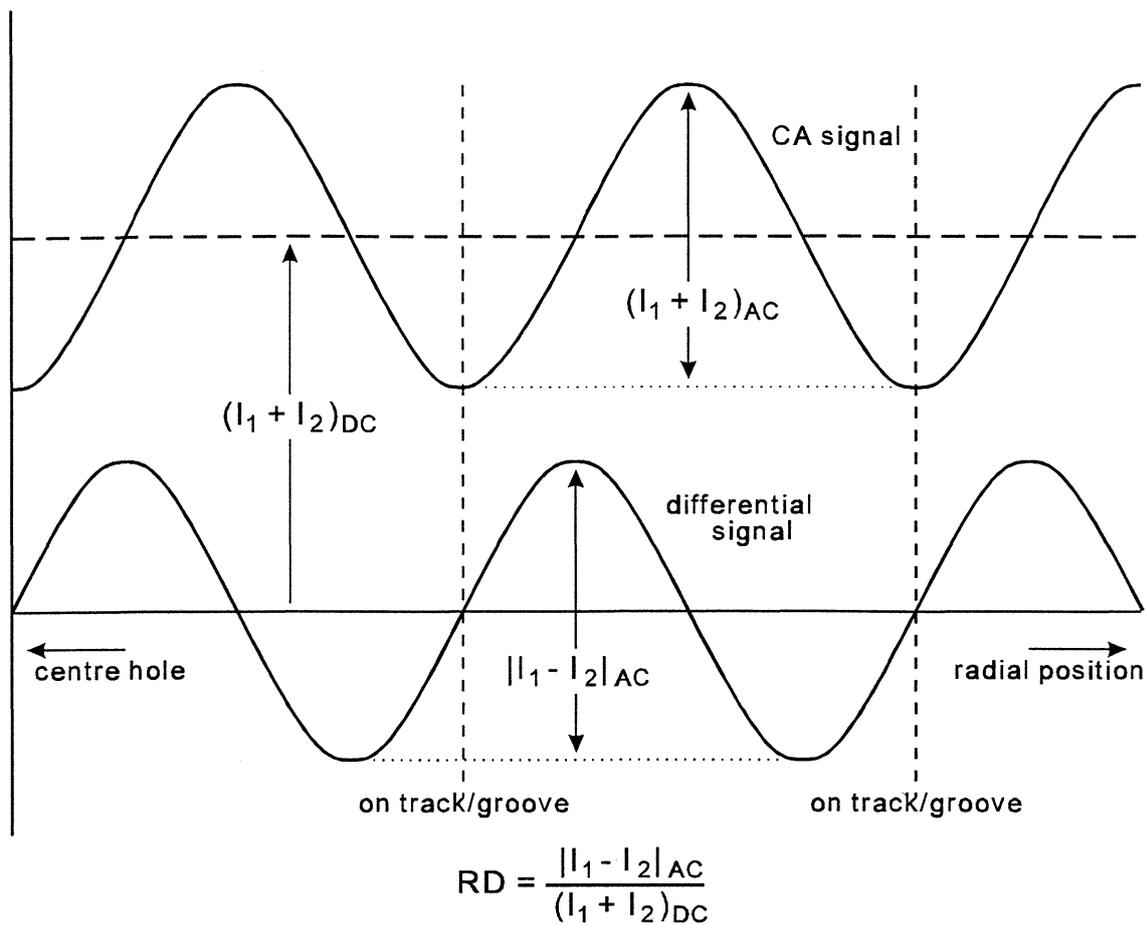
Figure II - 4.1 Definition of radial signals
