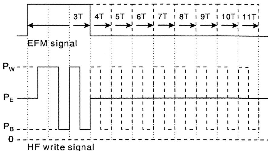
**Figure II - 1.2 Write strategy for 2x and 4x nominal CD speed**
