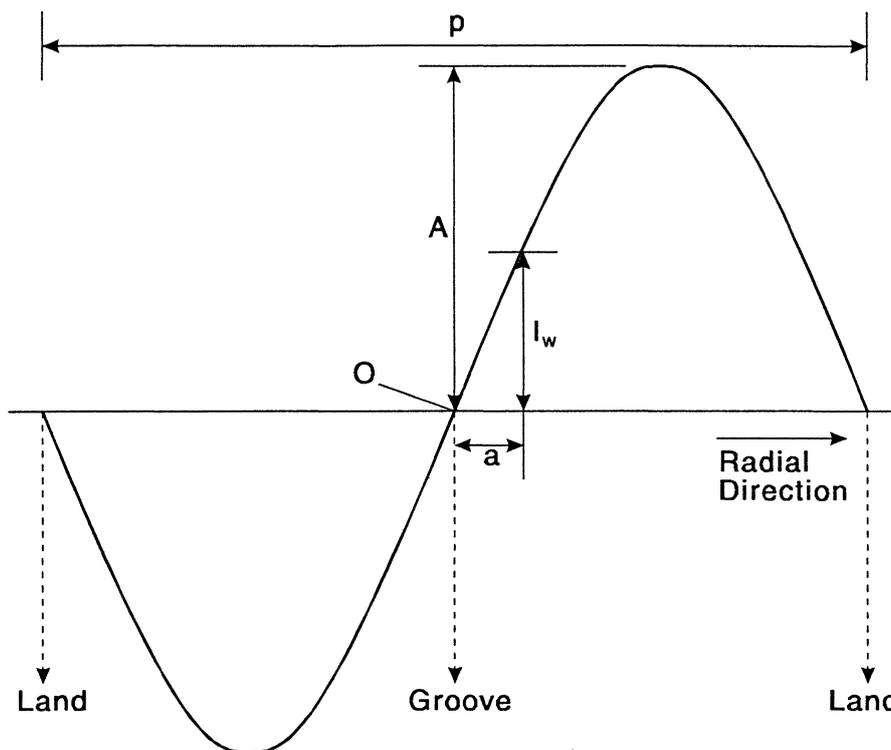
Figure C - 6.1 The radial error signal
