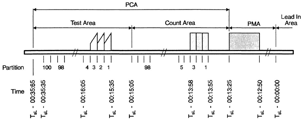
Figure V - 1 Organization of the PCA, PMA and Lead-In Area
