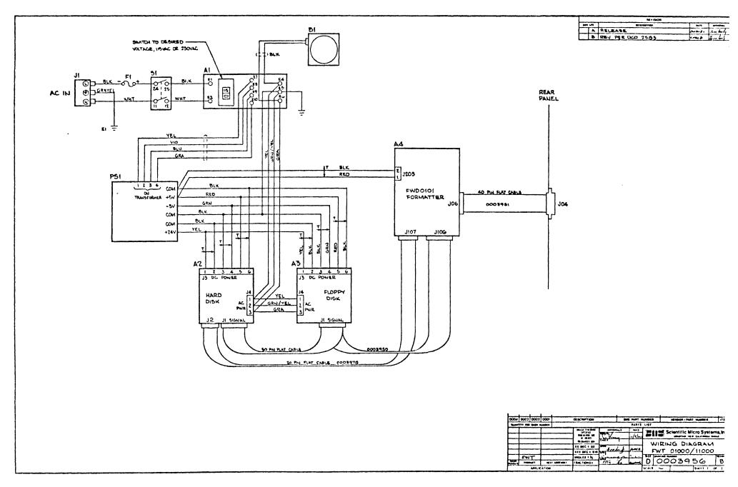
Figure 3. FWT System Wiring Diagram
