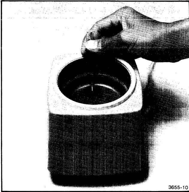
Figure E-9. Using the Ultrasonic Tank to Clean Pen Tips.
