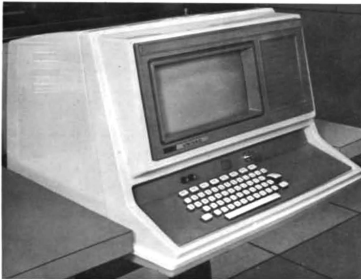
Figure 2-3. Keyboard and CRT Display Unit
