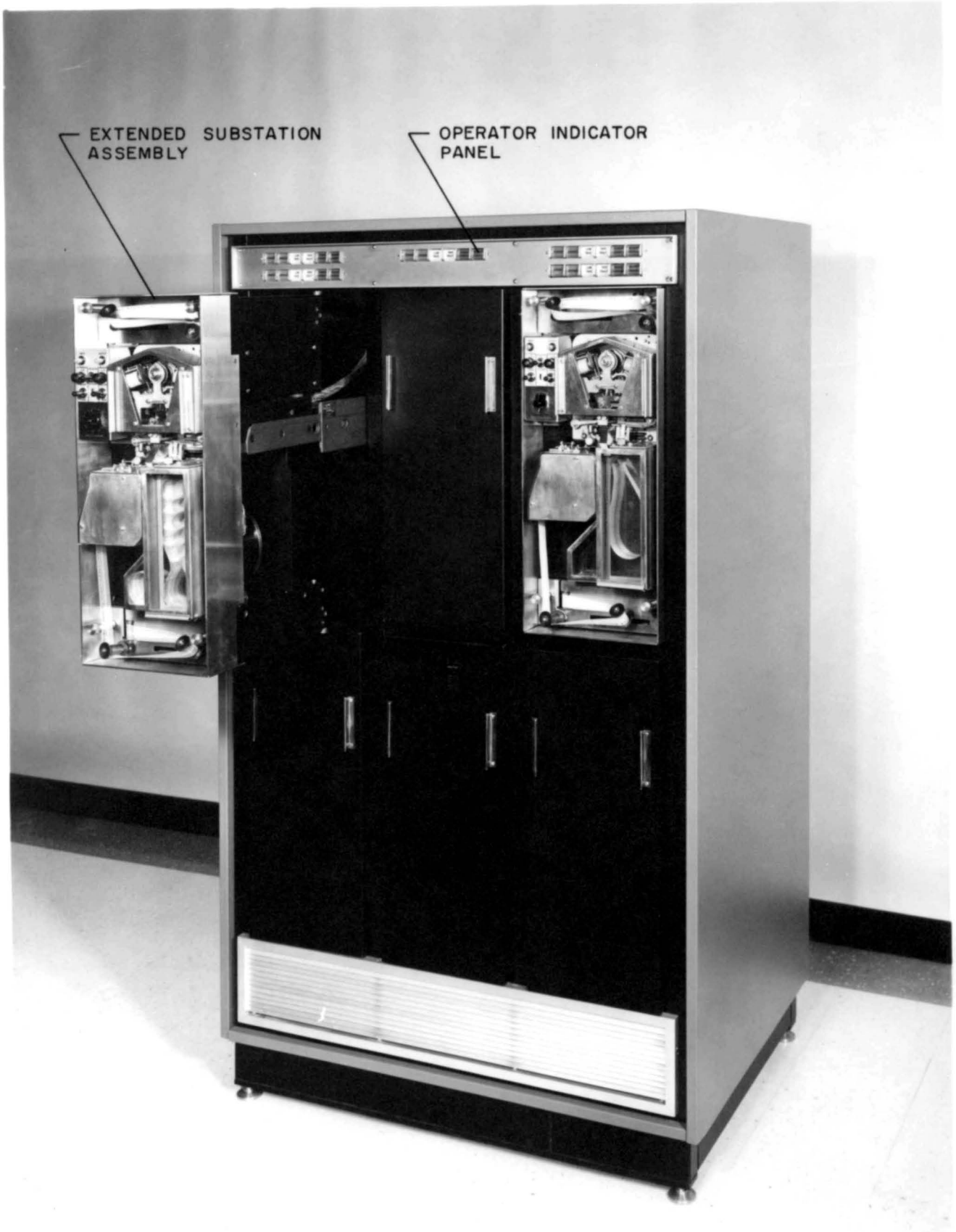
Figure 1-6. Substation Cabinet With One Substation Assembly Extended
