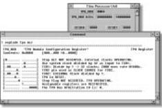
Using the Explode command, you can conveniently view register bit definitions on screen.
