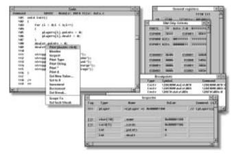
The MWX-ICE debugger speeds development with an intuitive, graphical interface that lets you perform tasks like setting breakpoints with a simple mouse click.
