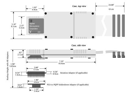
EL 3200 68360 Probe Tip and Adapter Dimensions
