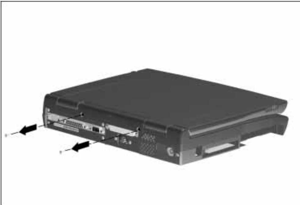
Figure 7-19. Removing the Microphone/Display Cable Cover Screws
