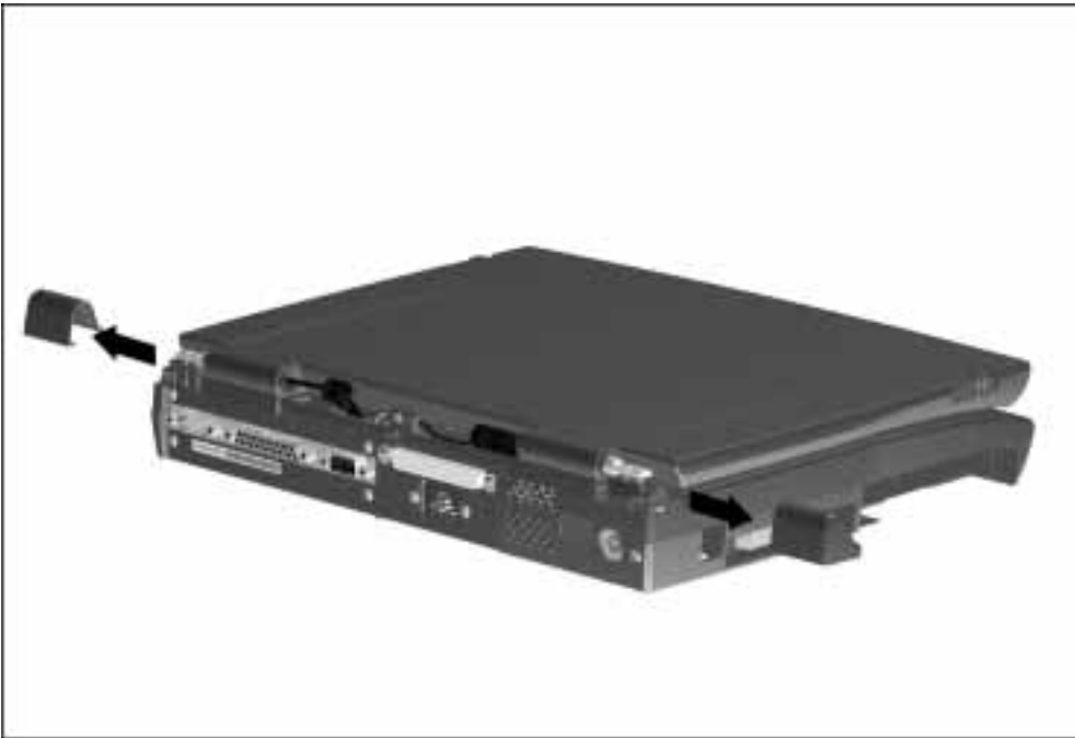
Figure 7-22. Removing the Clutch Covers
