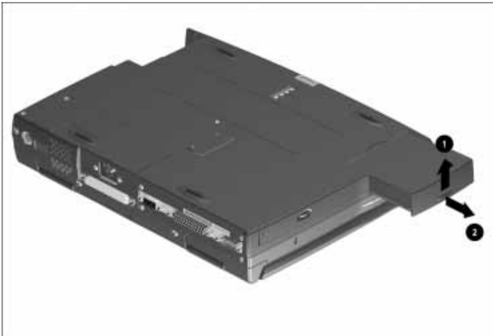
Figure 7-2. Removing the Battery Pack
