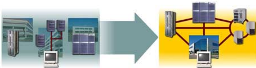
Figure 4: Illustrates the topology of transparent server consolidation
