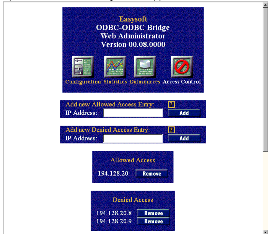
Figure 4.5: The Access Control Screen of the HTTP Interface
