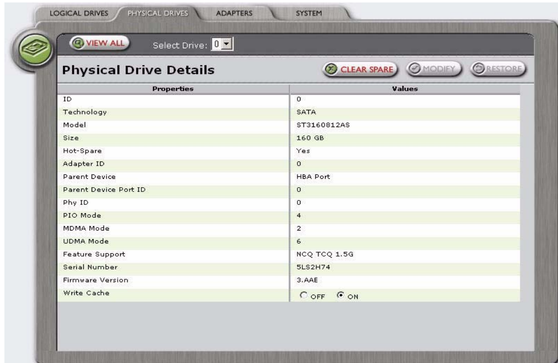
Figure 2-5 MRU Physical Drive Details
