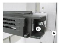
When you are done, the server should not slide on the channel bar.
