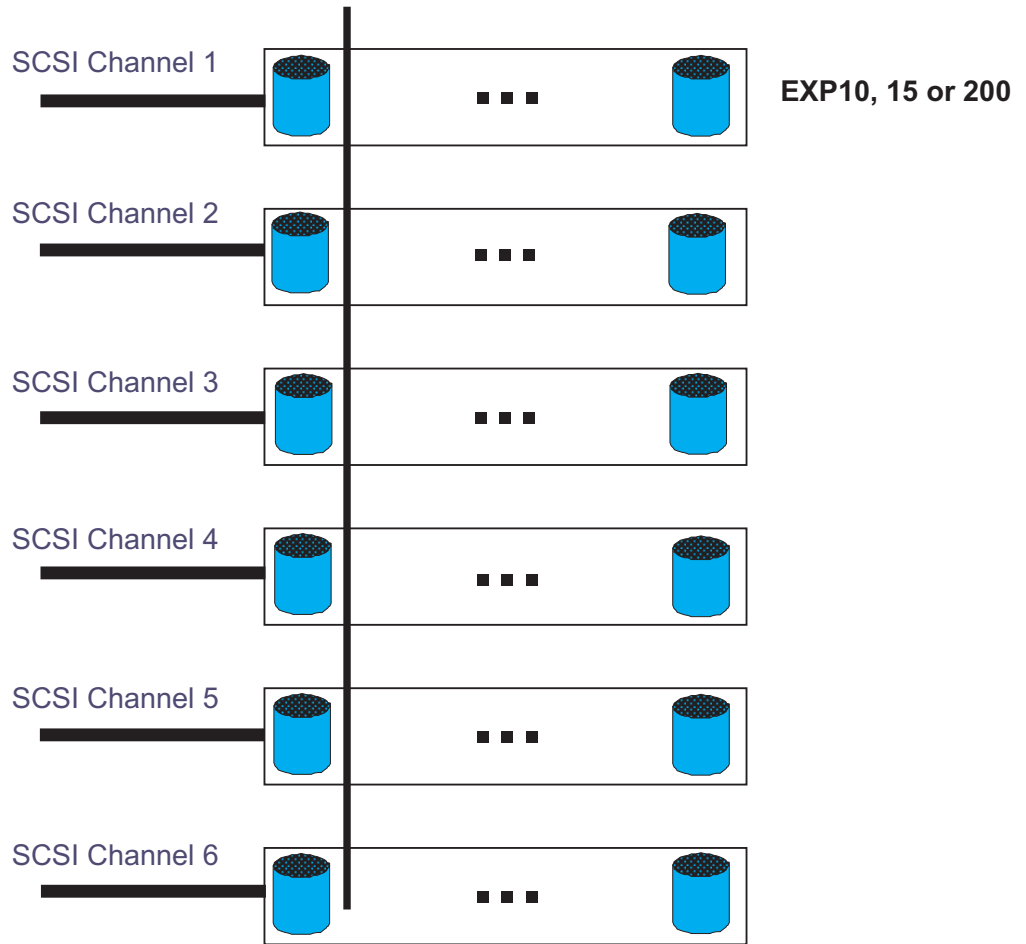
Figure 13. Type 3526 Fibre Channel RAID controller orthogonal data striping
